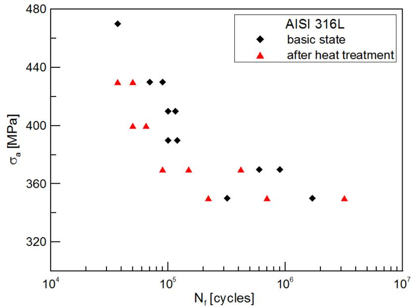
Fig. 4. Rotating bending fatigue tests results of AISI 316L in basic state and after structure sensitization. (full colour version available online)
