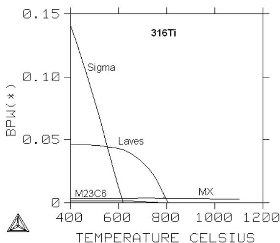
Fig. 1. Temperature dependence of weight fraction of minor phases in the steel 316Ti (ThermoCalc)
