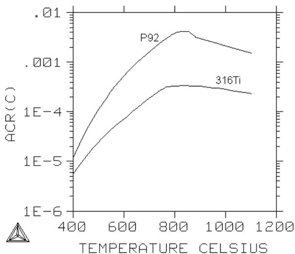
Fig. 7. Temperature dependence of activity for used steels (ThermoCalc calculation)
