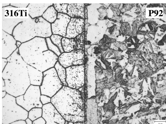
Fig. 4. Weld interface after annealing at 750°C/160h
