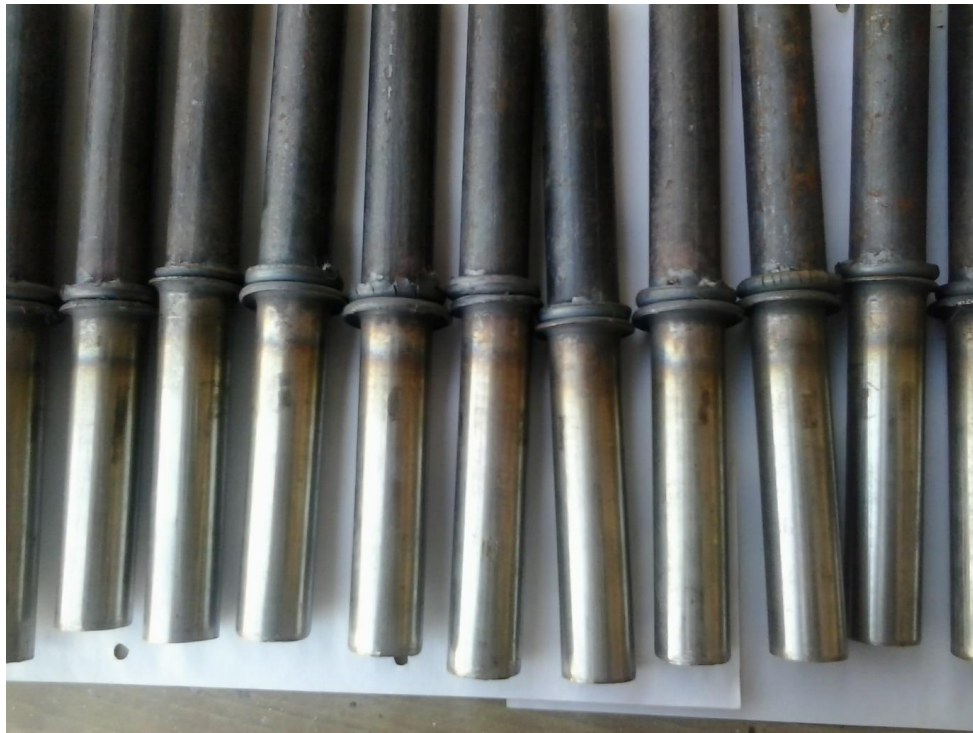
Fig. 1. Friction welded specimens. (full colour version available online)
