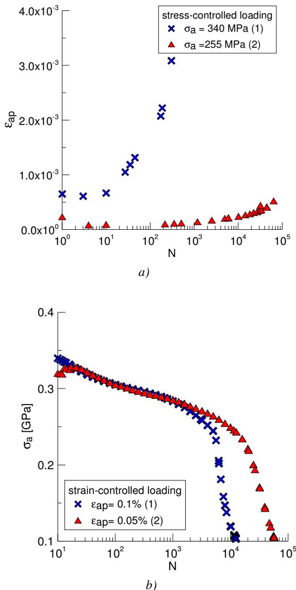
Fig. 3. Cyclic deformation response: a) stress-controlled and b) strain-controlled fatigue loading
