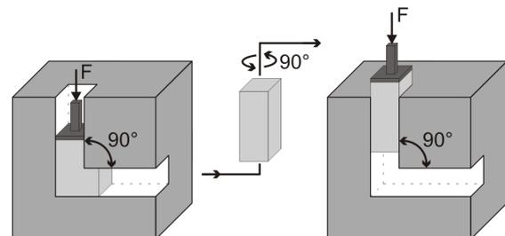
Fig. 1. Scheme of B<sub>C</sub> route of ECAP method
