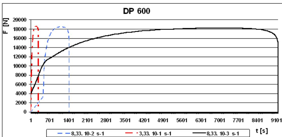
Fig. 4. Static tensile curves of DP 600 steels.
