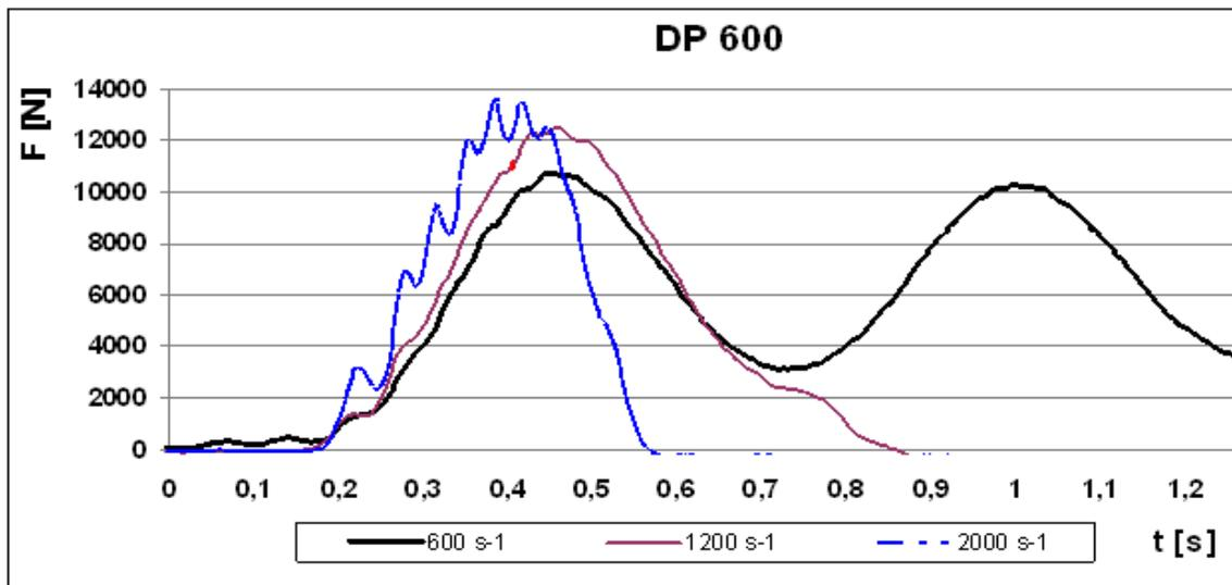
Fig. 5. Dynamic tensile curves of DP 600 steels.
