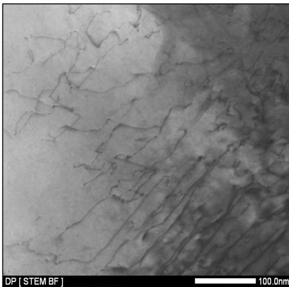
Fig. 6. Substructure of DP 600 steel in static conditions.
