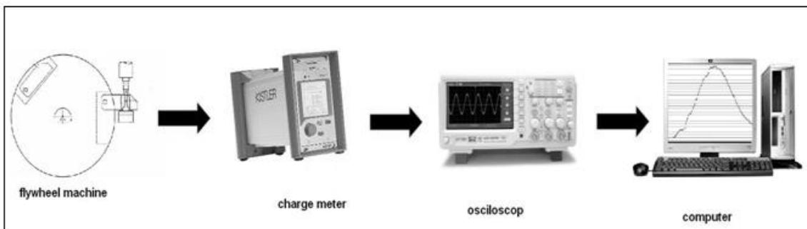
Fig. 2. Rotating wheel with a measurement system.
