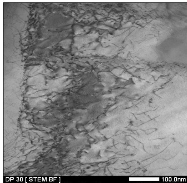
Fig. 7. Substructure of DP 600 steel in dynamic conditions.
