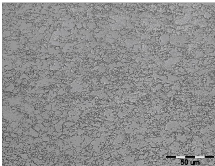
Fig. 3. Microstructure of DP 600 steel.
