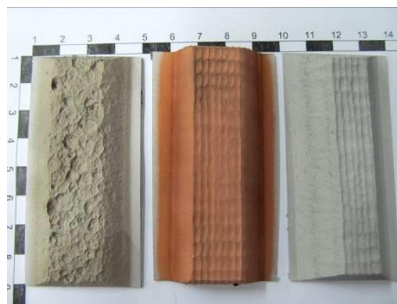
Fig. 3. As deposited bulk samples (NiFe, CuFe FeAl, from left to right). (full colour version available online)
