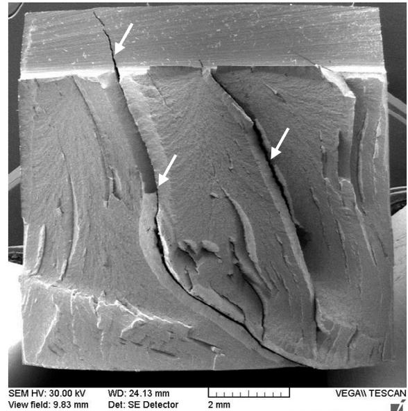
*Fig. 14. Fracture surface, damascus steel with 168 layers,  $T = 160\text{ }^{\circ}\text{C}$ ,  $KCU = 30.0\text{ J.cm}^{-2}$ , SEM*
