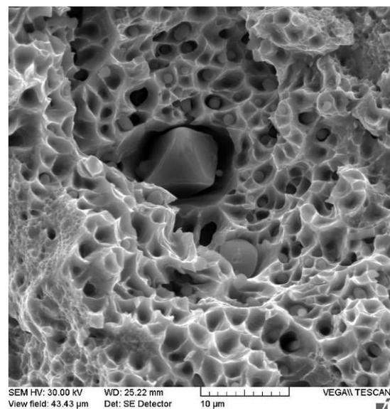
Fig. 7. Detail, welding layer, transcrystalline ductile fracture with expressive dimple morphology, damascus steel with 84 layers,  $T = 160^\circ\text{C}$ ,  $KCU = 15.6 \text{ J.cm}^{-2}$ , SEM
