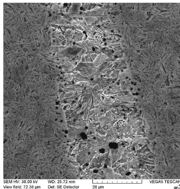
Fig. 2. Detail microstructure in the welding layer, SEM
