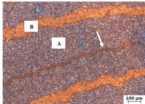
Fig. 1. Microstructure, damascus steel, light microscopy
