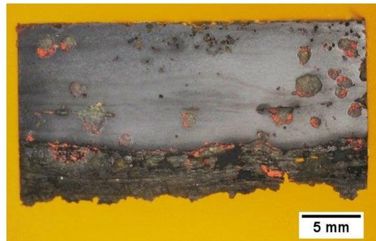
Fig. 18. Heyne etched longitudinal surface of knife 2 in polarized light.
