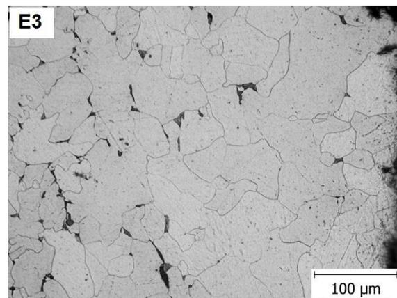
Fig. 14. Microstructure under surface of spine,
