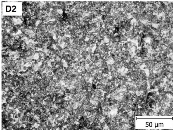
Fig. 15. Detail of edge, hardness 323 HV1.
