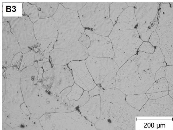
Fig. 9. Detail of middle part hardness 115HV1.
