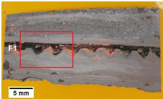
Fig. 17. Heyne etched longitudinal surface of knife 1 in polarized light.
