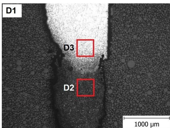
Fig. 11. Transition between spine to edge.
