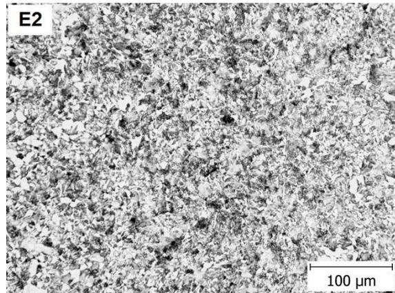
Fig. 16. Core of spine, hardness 197HV1.
