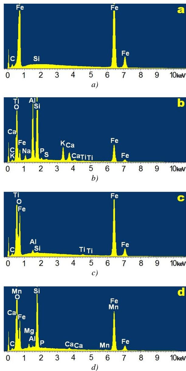
Fig. 25. Knife 2 EDX spectra: a) Spectrum of matrix, b) Spectrum of dark impurity, c) Spectrum of bright impurity, d) Spectrum of grey impurity.
