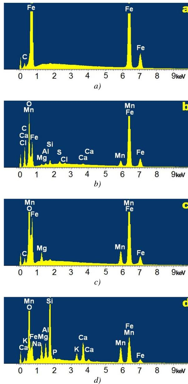
Fig. 23. Knife 1 EDX spectra: a) Spectrum of matrix, b) Spectrum of bright impurity, c) Spectrum of grey impurity, d) Spectrum of dark impurity.
