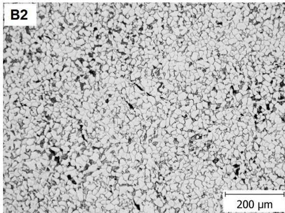
Fig. 7. Detail from spine, hardness 112HV1.
