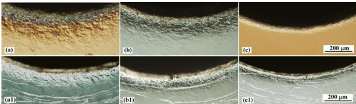
Fig. 4. Deformation zones (DZ) around the drilled hole observed on the surface of annealed samples: LC (a) MA-1 (b) and MA-2 steel (c). DZ observed on the surface of intercritically quenched samples: LC (a1), MA-1 (b1), and MA-2 steel (c1).
