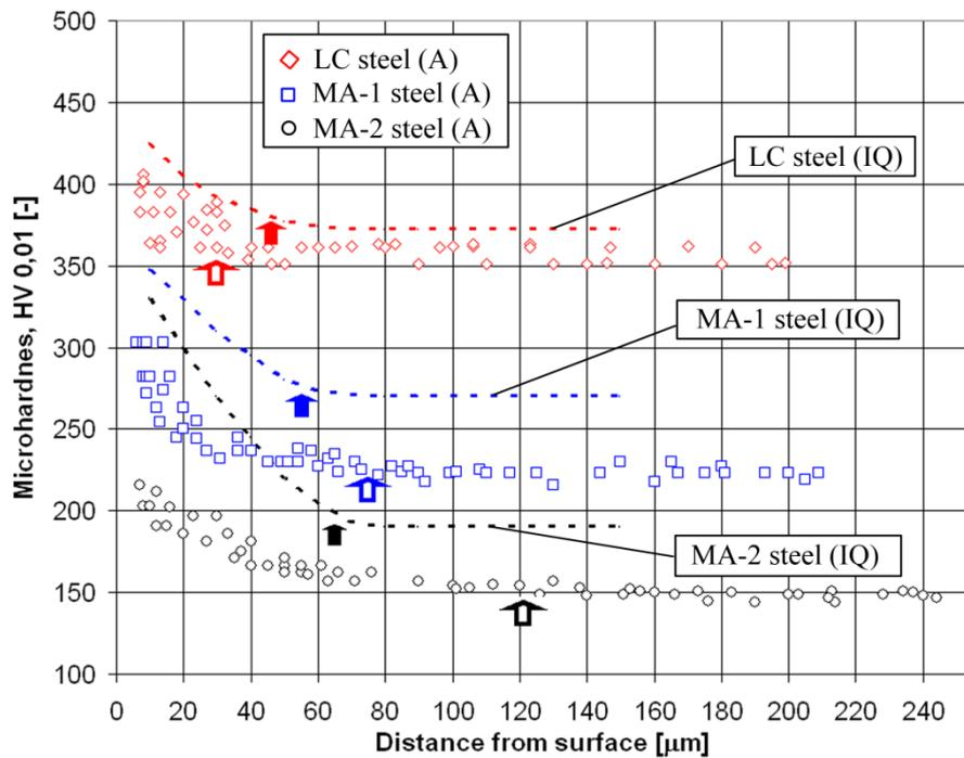
Fig. 3. Microhardness distribution profile near the surface of the drilled hole in LC, MA-1 and MA-2 steels measured on both annealed (A) and intercritically quenched (IQ) samples.
