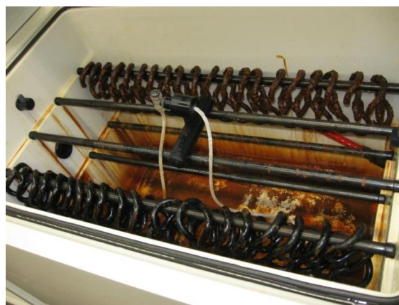
Fig. 2. The samples in corrosion chamber. (full colour version available online)
