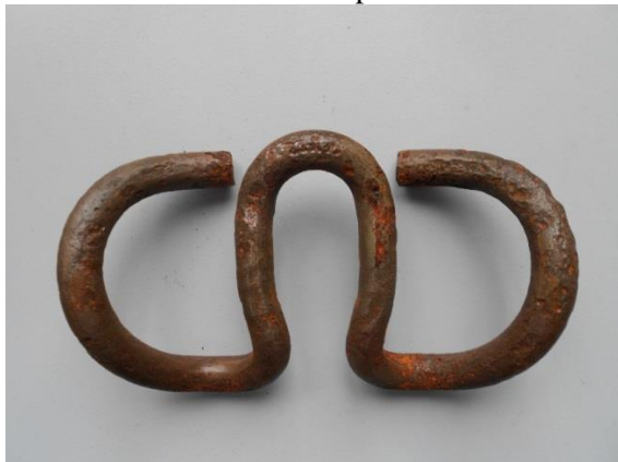
Fig. 4. The tension clamp without anticorrosion protection after corrosion loading. (full colour version available online)
