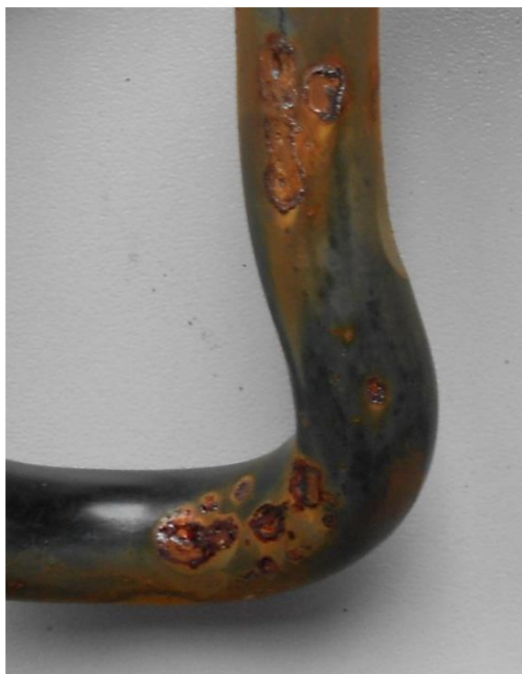
Fig. 6. The tension clamp with anticorrosion protection KTL after corrosion loading – detail of the corrosion. (full colour version available online)
