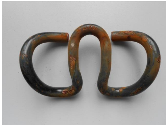
Fig. 5 The tension clamp with anticorrosion protection KTL after corrosion loading. (full colour version available online)
