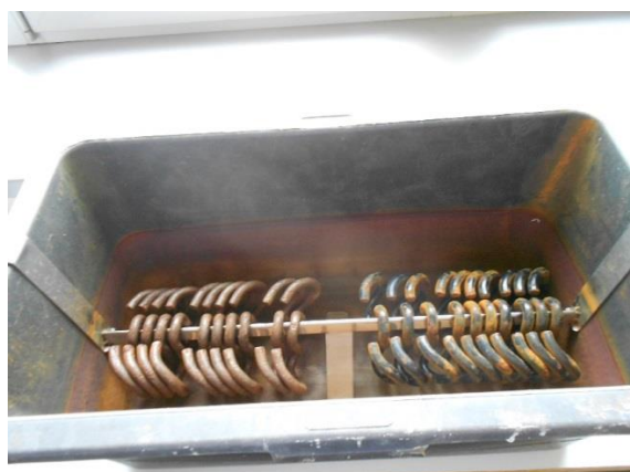
Fig. 3. The samples prepared for the immersion test in electrolyte solution. (full colour version available online)
