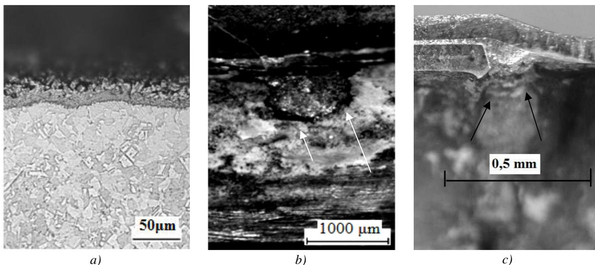
Fig. 5. Microstructure of the solder (a), detail of the soft solder pitting (b), pits close to the cross cut (c)
