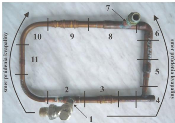
Fig. 1. The experimental cell with the marked joints and direction of corrosion medium flow
