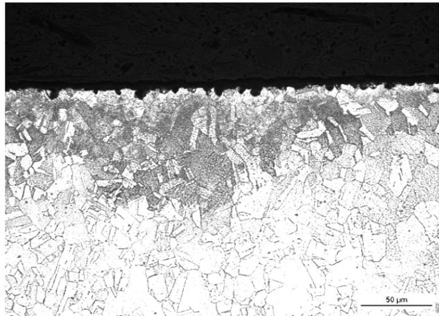
Fig. 3. Corrosion of the copper pipes after exposition in flowing solution
