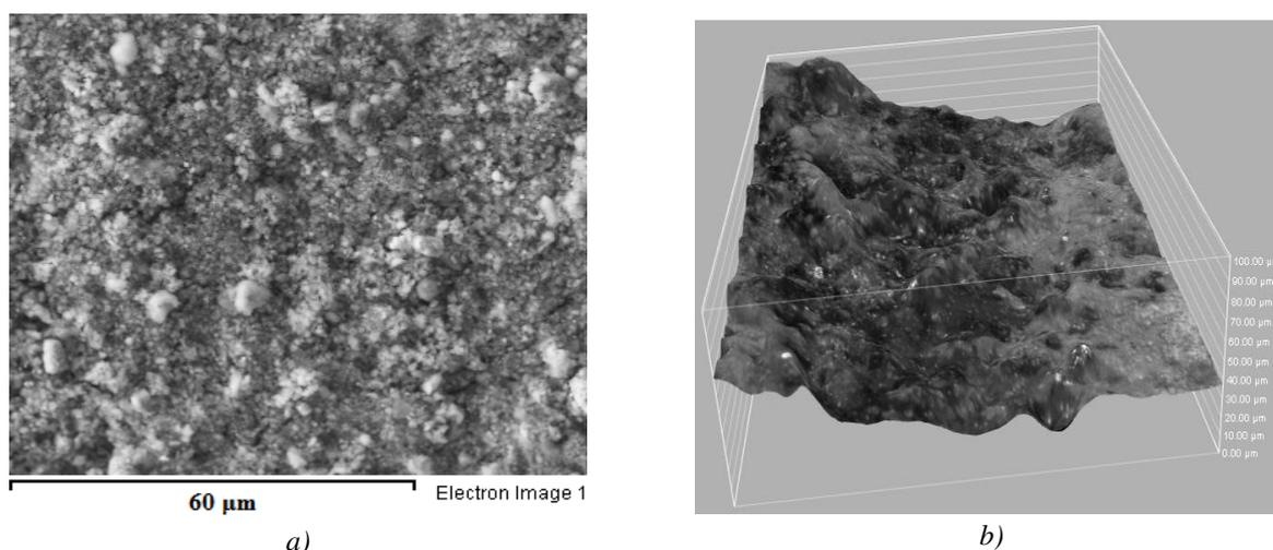
Fig. 6. Corrosion products (a) and soft solder surface morphology after exposition (b)
