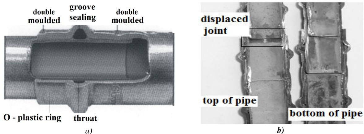
Fig. 7. Design of the fitting (a) and the state after the exposition (b)
