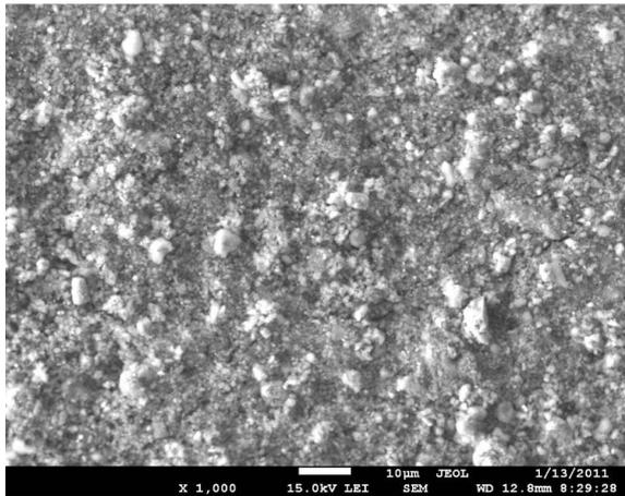
Fig. 2. Corrosion products on the surface of the copper pipes after the exposition in flowing solution
