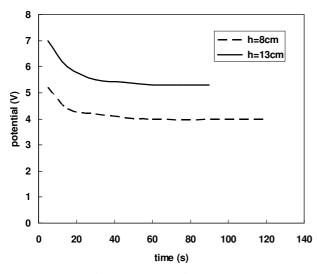
Fig. 7. Dependence of potential at constant current of 1A on time and distance (h) between the electric contact and electrolyte level
