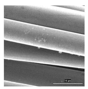
Fig. 6. Isolated Ni islands found on the surface of carbon fibres 190 mm below the electrolyte level after the 90 sec/1 A exposure
