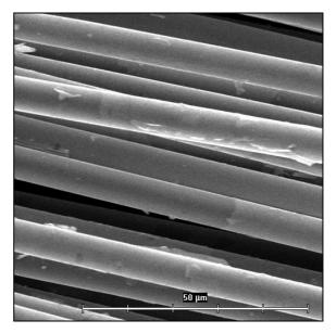
Fig. 2. Nickel coating formed just below the electrolyte level after the 15 sec/1 A exposure
