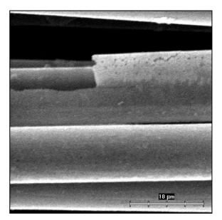
Fig. 5. Nickel coating formed just below the electrolyte level after the 90 sec/1 A exposure
