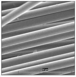
Fig. 1. Surface of original ASC4 carbon fibres
