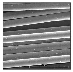
Fig. 3. Nickel coating formed 60 mm below the electrolyte level after the 15 sec/1 A exposure
