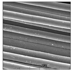
Fig. 4. Nickel coating formed 95 mm below the electrolyte level after the 15 sec/1 A exposure
