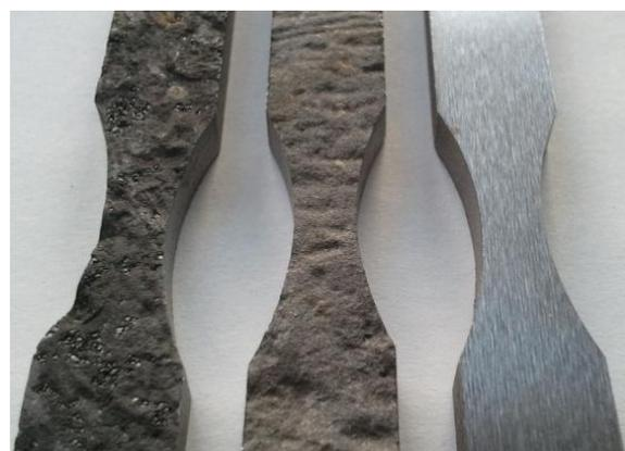
Fig. 3. Surface condition of specimens (from left as-cast, sand blasted, fine ground)
