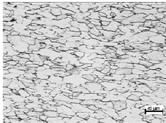
Fig. 4. Structure of wire behind the drawing die (place S5)
