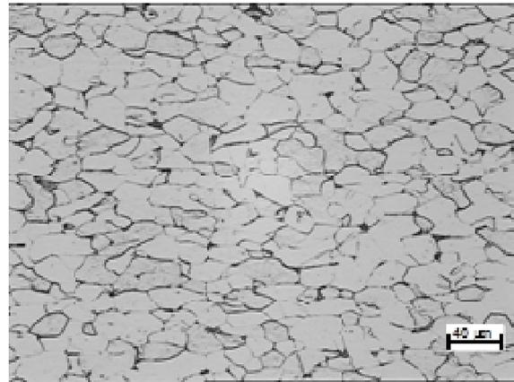
Fig. 3. Structure of wire in front of drawing die (place M1)
