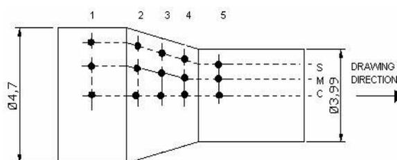
Fig. 1. Scheme of longitudinal section of the sample with places for the analysis
