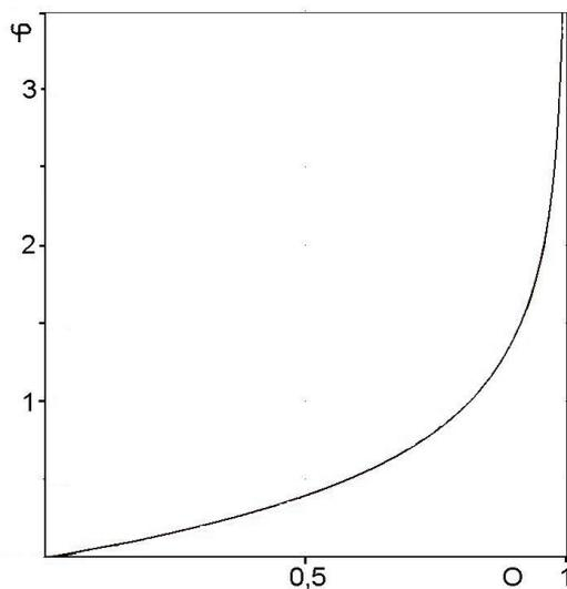
Fig. 2. Dependence of true strain to degree of grain boundary orientation [8]
