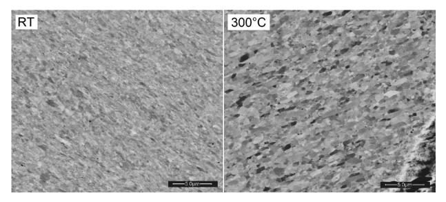
Fig. 7. SEM micrographs of the longitudinal section of 8x ECAPed sample deformed at room temperature and at  $300 \ ^{\circ}C$
