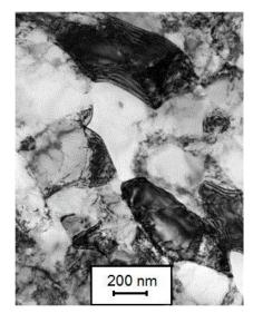
Fig. 2. TEM micrograph of the cross section of 8x ECAPed sample
