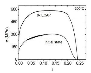
Fig. 6. Comparison of true stress-true plastic strain of initial state and 8x ECAPed samples, respectively, at 300  $^{\circ}C$
