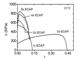
Fig. 5. True stress-true plastic strain curves at 21 °C obtained for various numbers of ECAP passes
