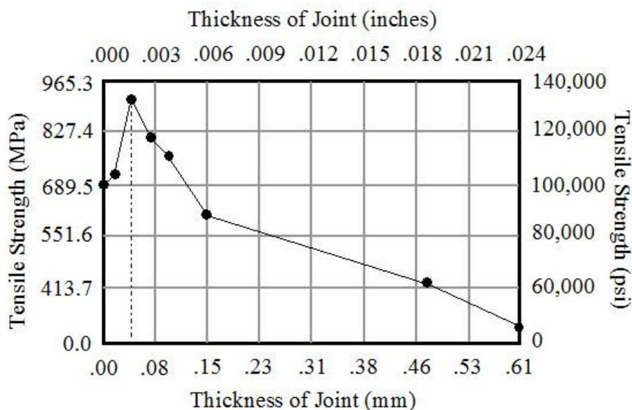
Fig. 1. Effect of joint clearance on tensile strength.
