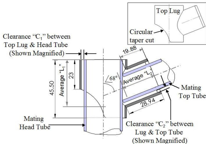
Fig.19. Volume of brass layer in top lug joint.
