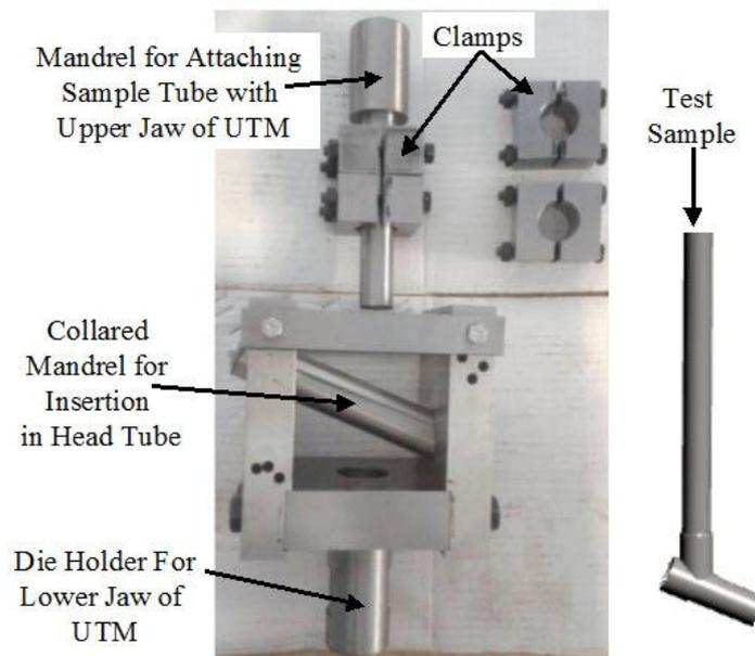
Fig. 15. Testing fixture and test sample for use on universal testing machine.
