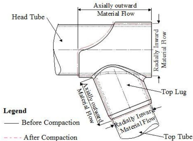
Fig. 13. Flow of materials during compaction.
