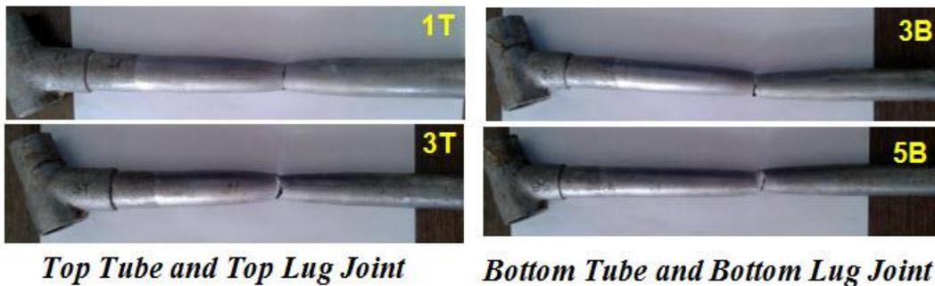
Fig. 16. Brazed joint samples tested on universal testing machine.
