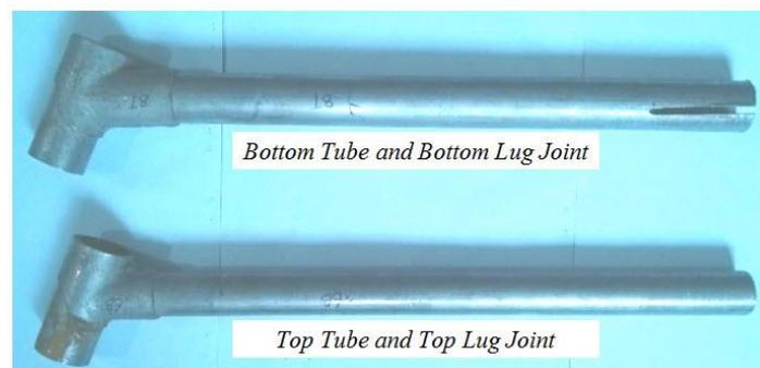
Fig. 14. Samples of joints for testing of tensile strength on universal testing machine.
