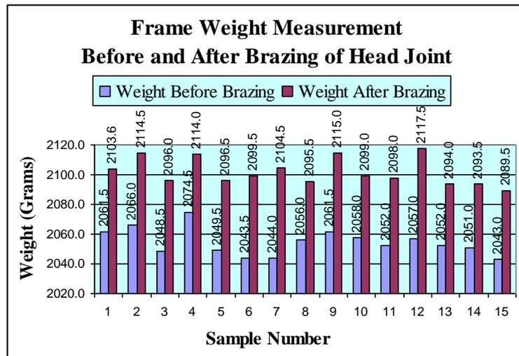
a) frame weight measurement - before and after brazing of head joint
