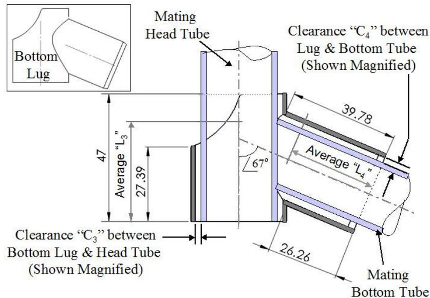
Fig. 20. Volume of brass layer in bottom lug joint.
