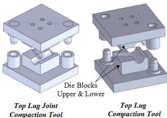
Fig. 11. Compaction press tools for head parts.
