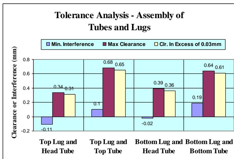
Fig. 5. Tolerance analysis - assembly of tubes and lugs.
