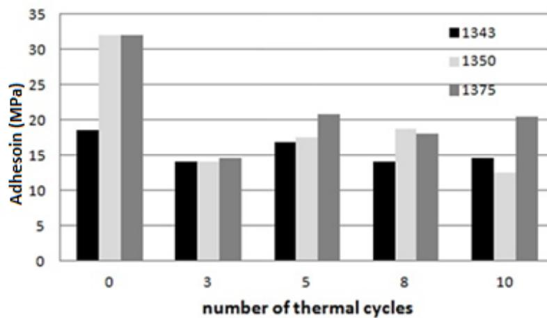
Fig. 3. Adhesive wear of coatings after thermal cycles.
