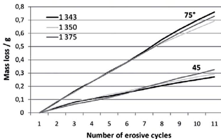
Fig. 4. Erosive wear of the coatings [4].
