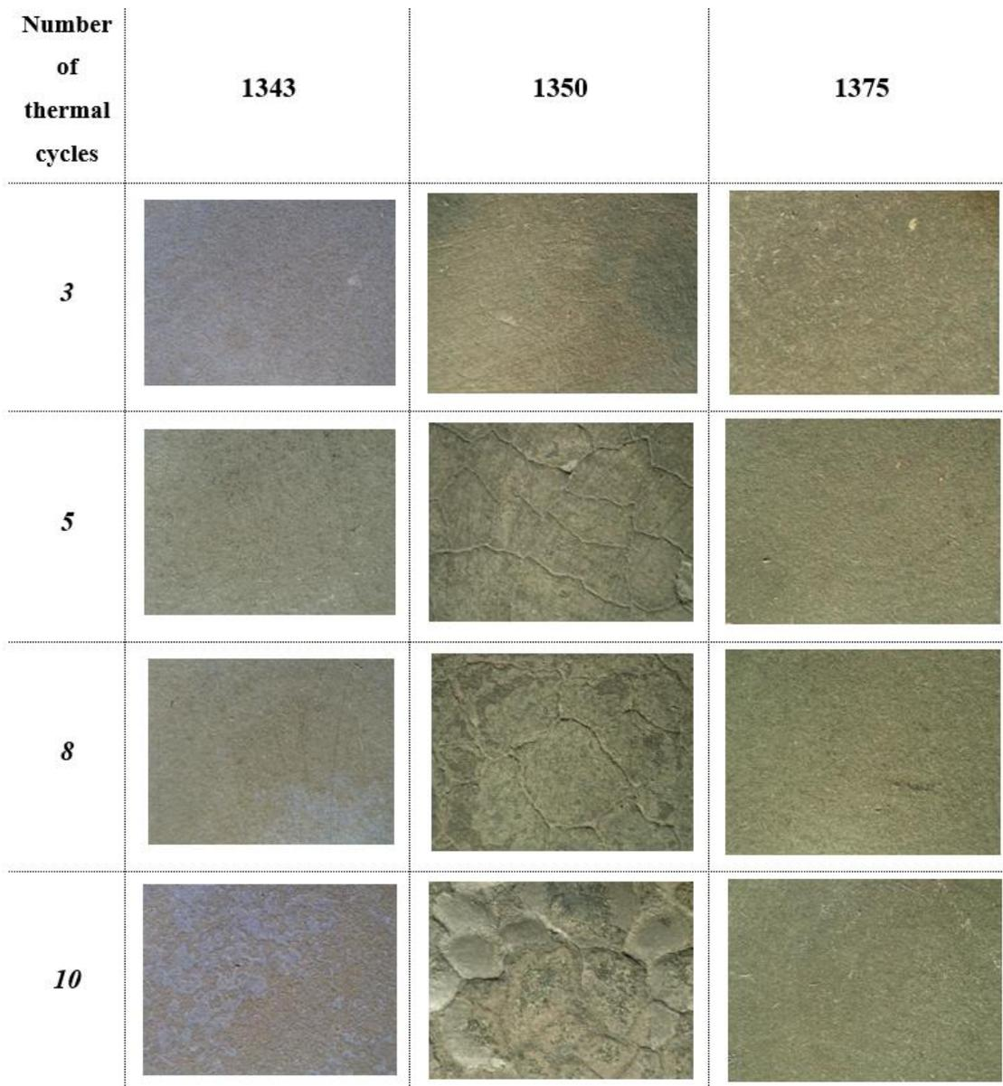
Fig. 5. Appearance of surfaces of investigated coatings after thermal cyclic loading [8].
