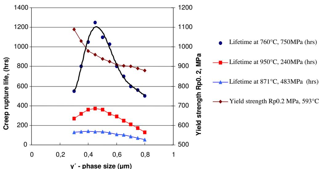
Fig. 9. Gamma prime size and its influence on chosen mechanical characteristics at various temperatures
