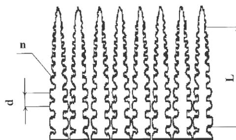
Fig. 3. Scheme for secondary dendrite arm spacing evaluation
