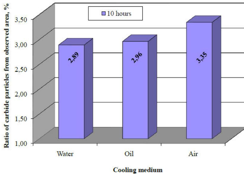
Fig. 5. Ratio of carbide particles from observed area
