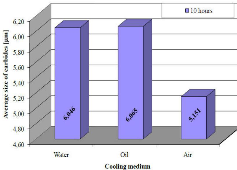
Fig. 6. Average carbides size (μm)
