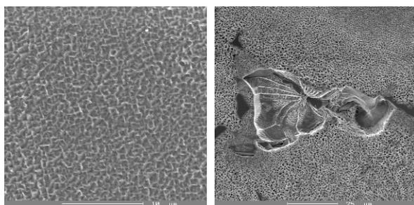
a) matrix and  $\gamma$  phase      b)  $\gamma/\gamma'$  eutectic
