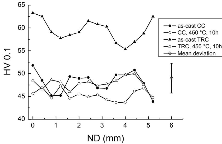
Fig. 3. Evolution of inhomogeneity in AZ31 magnesium alloys during heat treatment.
