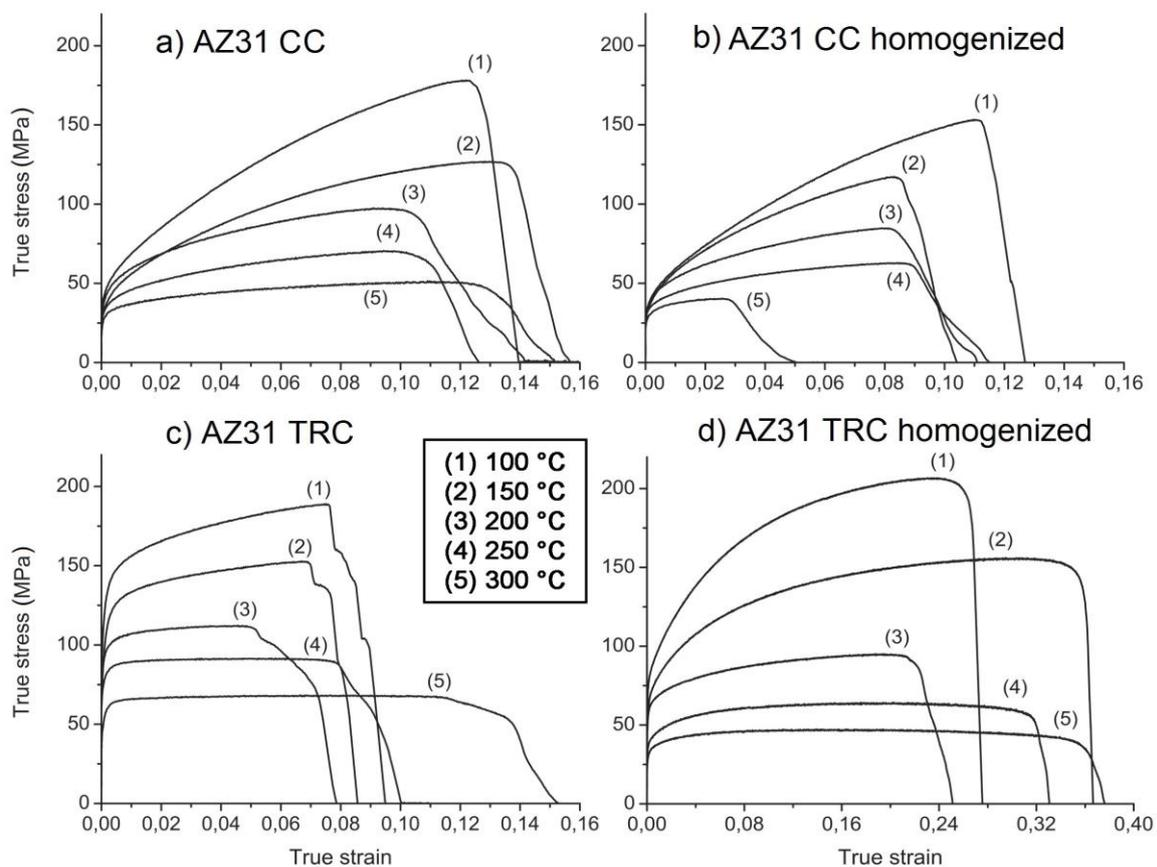
Fig. 5. Stress-strain curves for AZ31 magnesium alloys during annealing at temperature range from 100 °C – 300 °C: a) as-cast CC, b) CC after homogenization annealing at 450 °C for 10 hours, c) as-cast TRC, d) TRC at 450 °C for 10 hours (note the scale on the figure 5d).
