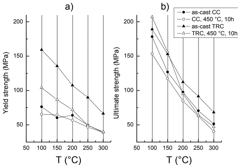
Fig.6. Temperature dependence of the yield (a) and ultimate (b) strengths of the conventionally cast and twin-roll cast AZ31 magnesium alloys before and after aging at 450 °C for 10 h.
