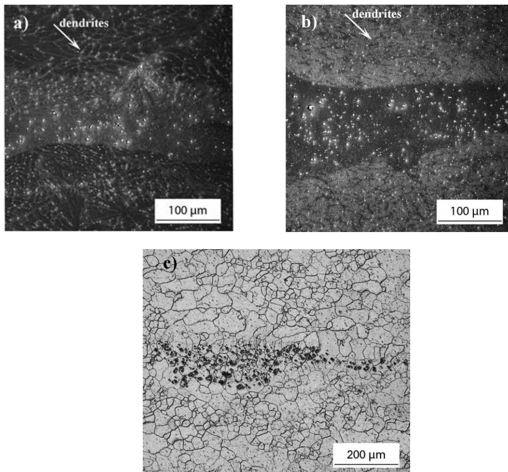
Fig. 2. SEM images of the dendritic structure and central segregation zone in TRC AZ31 magnesium alloy: a) as-cast, b) after aging at 450 °C for 10 h and c) image made by light microscope after aging at 450 °C for 10 h.
