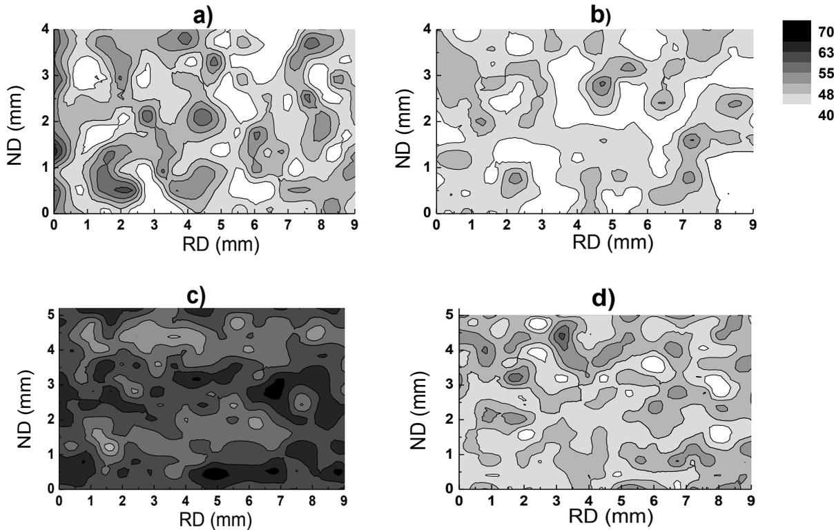
Fig. 4. Microhardness mapping (in MPa) of the cross-section of AZ31 magnesium alloys: a) as-cast CC AZ31 alloy, b) CC alloy after homogenization annealing at 450 °C for 10 h, c) as-cast TRC alloy, d) TRC alloy after homogenization annealing at 450 °C for 10 h.
