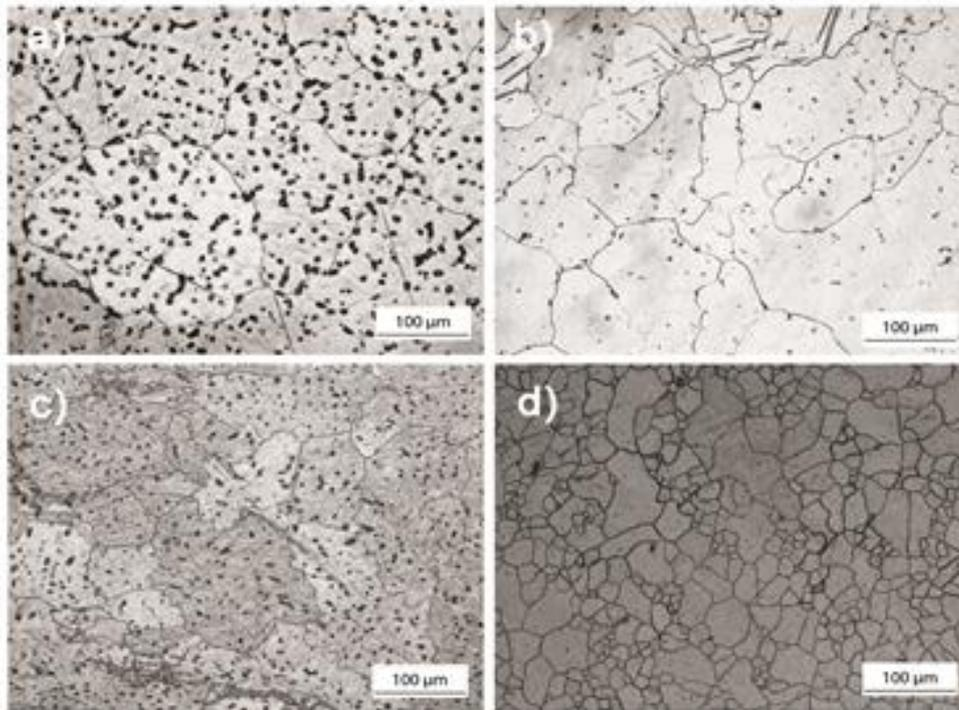
Fig. 1. Microstructure of AZ31 magnesium alloys: a) CC as-cast, b) CC after homogenization annealing at 450 °C for 10 hours, c) TRC as-cast, d) TRC after homogenization annealing at 450 °C for 10 hours.
