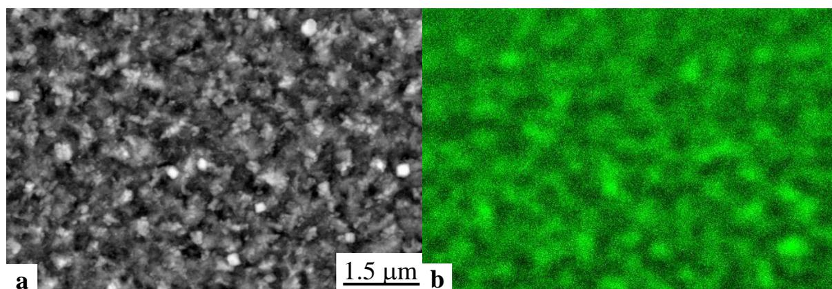
Fig. 3. SEM micrograph showing (a) the surface microstructure of CrAg15N – film and (b) corresponding EDS-map of silver
