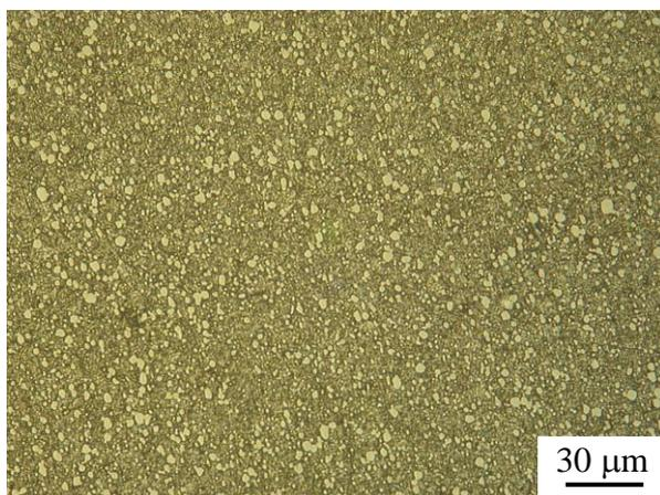
Fig. 1. Microstructure of PM ledeburitic steel Vanadis 6 substrate after heat treatment
