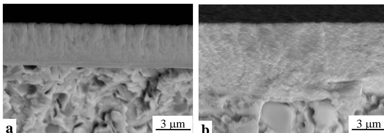
Fig. 2. SEM micrographs showing: (a) the microstructure of CrAg3N and (b) CrAg15N films developed on the Vanadis 6 steel substrate
