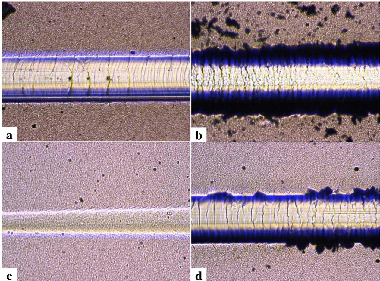
Fig. 4. Light micrographs showing the failures after scratch test: a – CrAg3N,  $L_{c1}$ , b – CrAg3N,  $L_{c2}$ , c – CrAg15N,  $L_{c1}$ , d – CrAg15N,  $L_{c2}$
