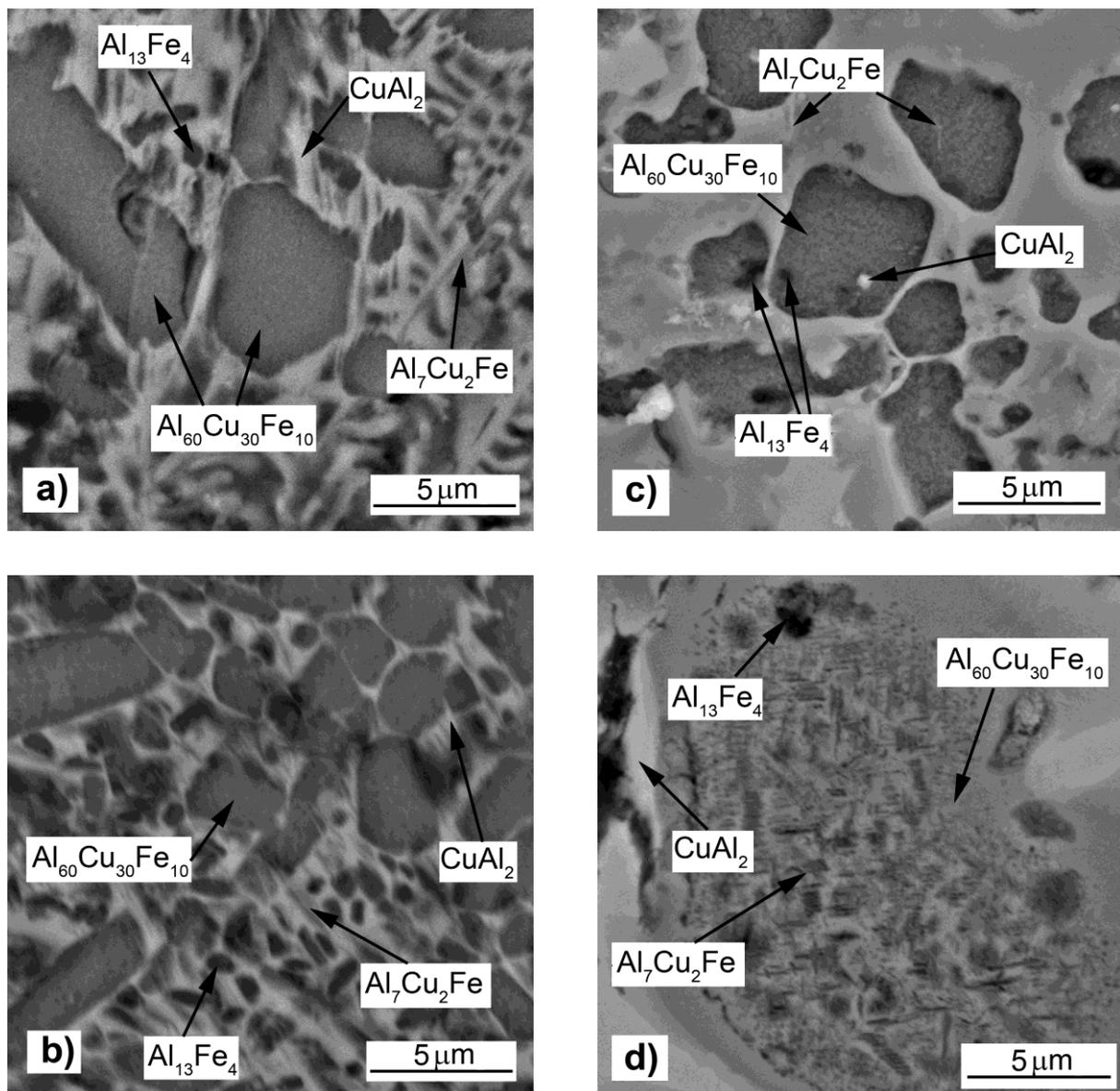
Fig. 5. Microstructure (SEM) of the material prepared by SHS and annealed at a) 300°C for 4 h, b) 300°C for 40 h, c) 500°C for 4 h and d) 500°C for 40 h
