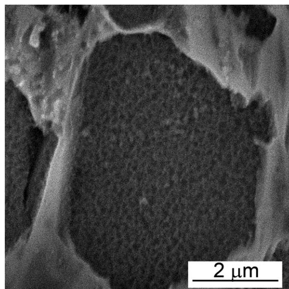
Fig. 4. Detail of the microstructure (SEM) of the material prepared by SHS and water cooling.
