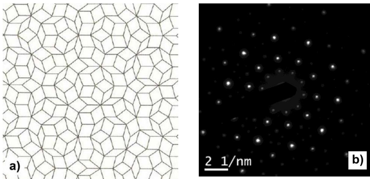
Fig. 1. a) Penrose tiling, b) diffraction pattern of Al-Cr-Fe quasicrystalline phase [1]
