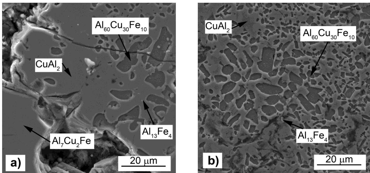
Fig. 3 Microstructure (SEM) of the material prepared by SHS and a) air cooling, b) water cooling
