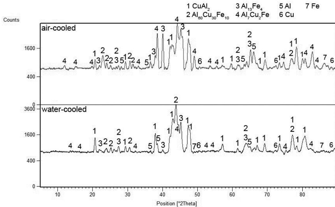
Fig. 6. XRD patterns of Al-Cu-Fe alloy prepared by SHS process followed by water cooling, annealed at 400 and 500°C for 4 and 40 h
