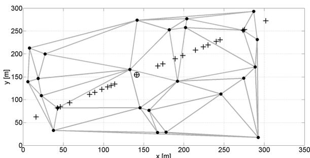
Fig. 4: The original end-points and their projections on a minimum line with the position of a central splitter marked by a circle.
