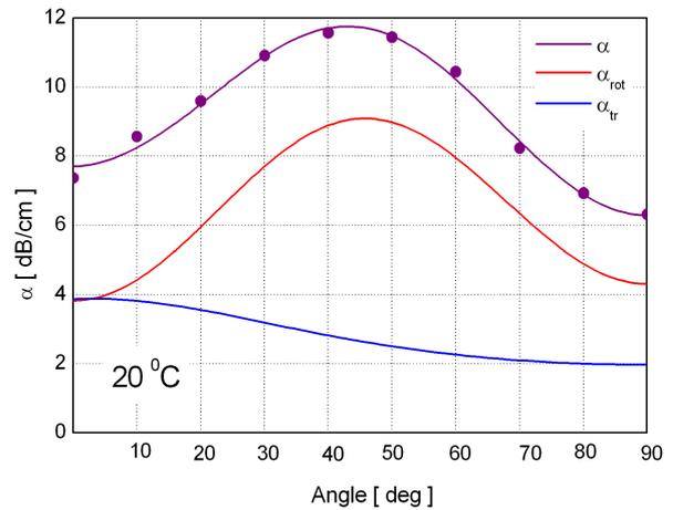
**Fig. 5:** Anisotropy measurement of the acoustic attenuation in external magnetic field 200 mT at the temperature 20 °C in the 2 % MF and the components  $\alpha_{rot}, \alpha_{tr}$  from the Taketomi theory [12].
