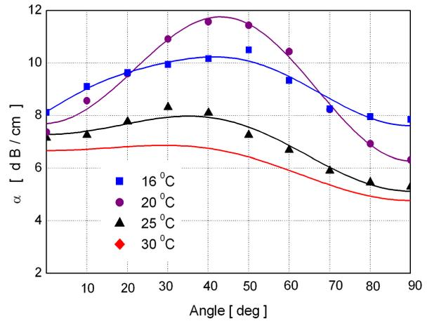
**Fig. 4:** Anisotropy measurement [15] of the acoustic attenuation at 200 mT external magnetic field in the 2 % MF and sum of the components  $\alpha_{rot} + \alpha_{tr}$  of the Taketomi functions [10] (blue 16 °C, violet 20 °C, black 25 °C, red 30 °C).
