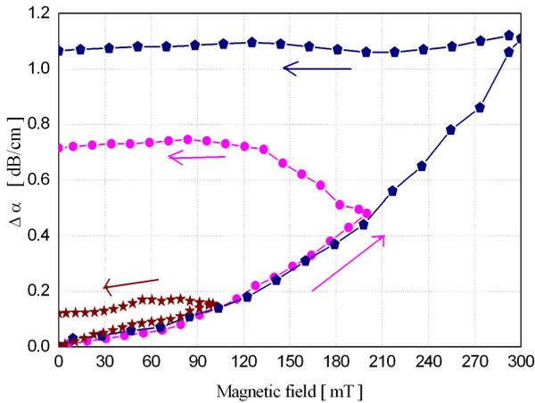
**Fig. 2:** Changes of the acoustic attenuation in external magnetic field for 2,5 % MF measured at 20 °C for different achieved maximum values of magnetic field (red - 100 mT, pink - 200 mT, blue - 300 mT). Magnetic field increased and/or decreased at a constant rate, 2,2 mT/min.
