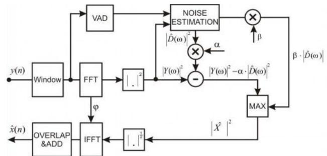
Fig. 3: Block diagram of modified spectral subtraction.
