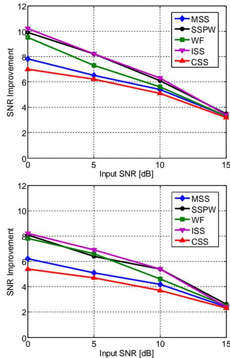
Fig. 5: SNR improvement of noise reduction algorithms for (a) AWGN noise, (b) Car noise.
