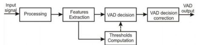
Fig. 2: Block diagram of a basic VAD design.
