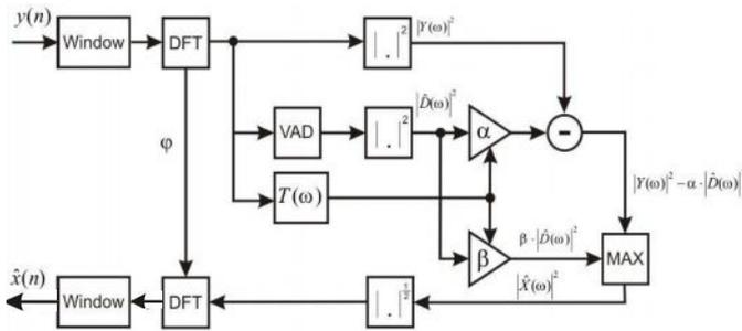
Fig. 4: Block diagram of a spectral subtraction with perceptual weighting.
