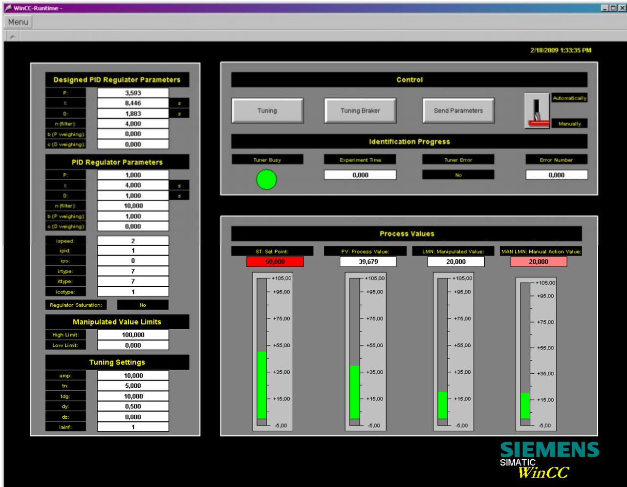
Fig. 9: The visualization of the moment self tuner.
