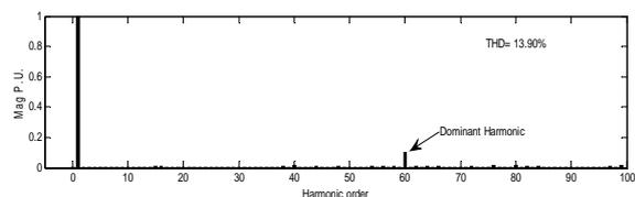
Fig. 6: Pole voltage THD  $m_f = 60, f_c = 3$  kHz.
