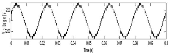
Fig. 10: Line voltage  $f_c = 1$  kHz.
