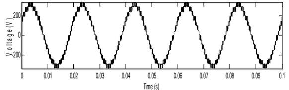
Fig. 13: Line voltage  $f_c = 2$  kHz.
