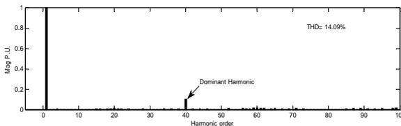
Fig. 5: Pole voltage THD  $m_f = 40, f_c = 2$  kHz.
