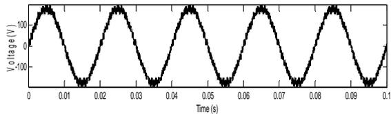
Fig. 18: Phase voltage  $f_c = 4$  kHz.
