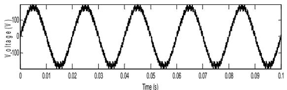
Fig. 15: Phase voltage  $f_c = 3$  kHz.
