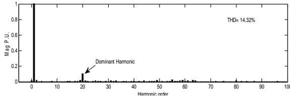
Fig. 4: Pole voltage THD  $m_f = 20, f_c = 1$  kHz.
