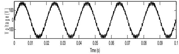
Fig. 12: Phase voltage  $f_c = 2$  kHz.
