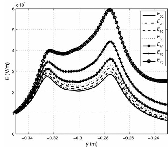
Fig. 5. Distribution of the module of electric field strength  $|\mathbf{E}|$  along line AB (see Fig. 4) for different positions of the knife
