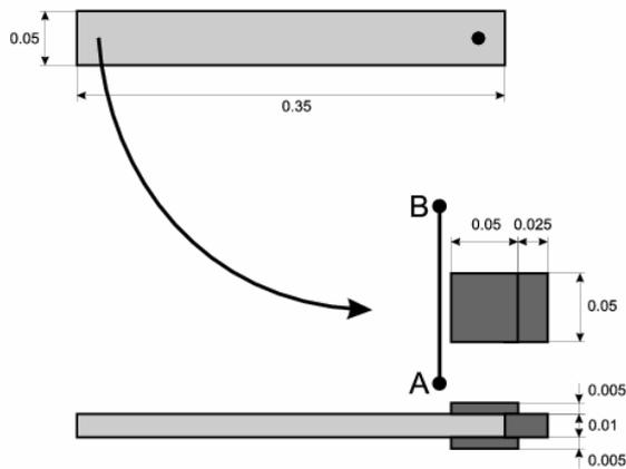
Fig. 3. Details of both contacts of the disconnector
