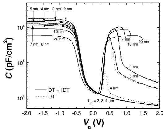
Fig. 4 Capacitance curves of the Ru/Ta<sub>2</sub>O<sub>5</sub>/SiO<sub>2</sub>/Si(p) structure for variable thickness of the oxide layer.
