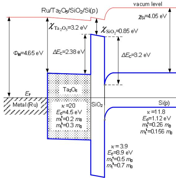
Fig. 2 Band diagram of a Ru/Ta<sub>2</sub>O<sub>5</sub>/SiO<sub>2</sub>/Si(p) MOS structure with material parameters.
