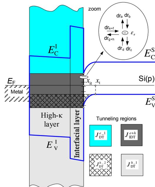
Fig. 1 Band diagram of a MOS structure showing the boundaries for calculation of tunnelling currents.
