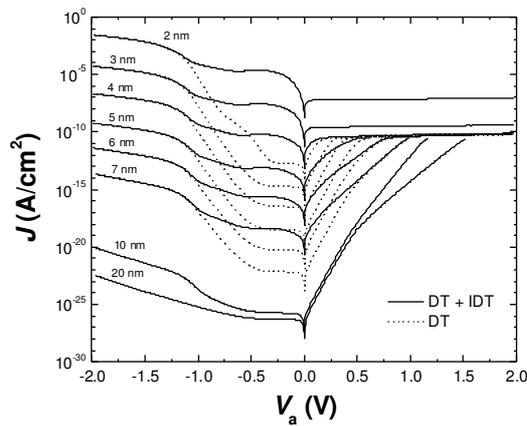
Fig. 3 Current densities through Ru/Ta<sub>2</sub>O<sub>5</sub>/SiO<sub>2</sub>/Si(p) structure for various thicknesses of the oxide layer.
