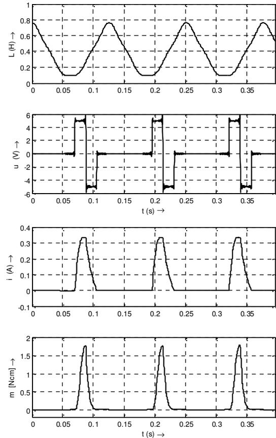
Fig.5. Waveforms of the electrical quantities in motoring
