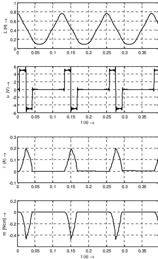
Fig.6. Waveforms of the electrical quantities in generating
