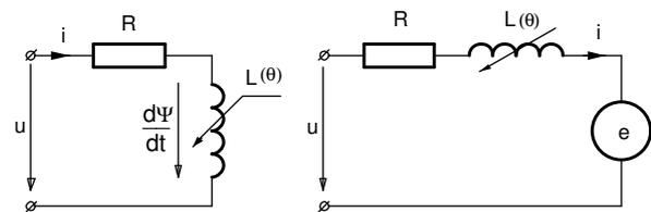
Fig. 2. Equivalent circuit of reluctance motor
