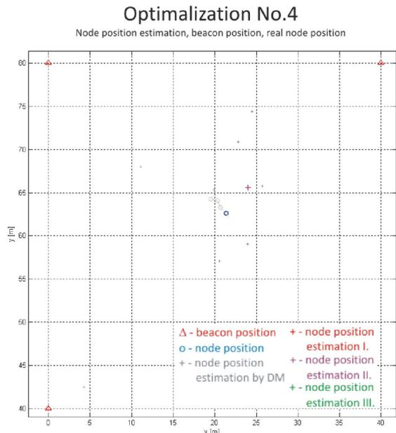
Fig. 8. On this figure is shown second step, where beacons were reduced from 4 to 3.
