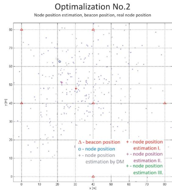
Fig. 6. On this figure is shown second step, where beacons were reduced from 9 to 6.
