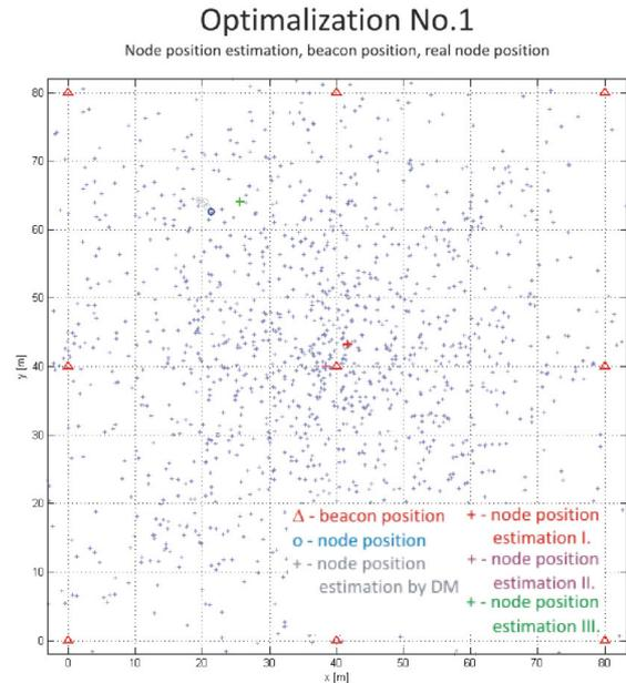
Fig. 5. In this case was beacons organised in grid and unknown mobile node was moved in four hops.
