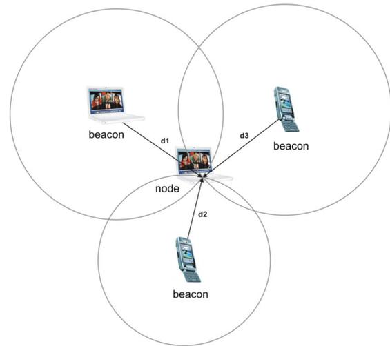
Fig. 3. Practical demonstration of trilateration in mobile ad-hoc networks.
