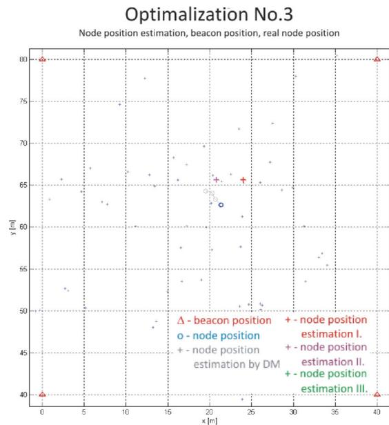
Fig. 7. On this figure is shown second step, where beacons were reduced from 6 to 4.
