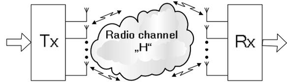
Fig. 2. The principle of MIMO channel
