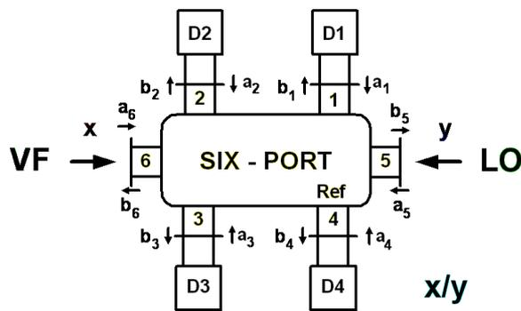
Fig. 1. Principle of the SPR [1]
