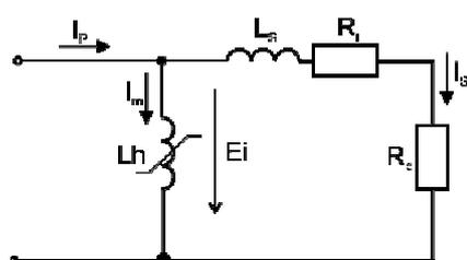
Fig. 1. One phase model of a CT
