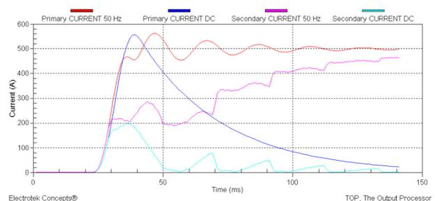
Fig. 9. Components of the primary and secondary currents
