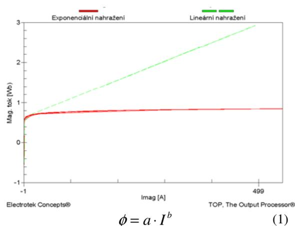
Fig. 2. Exponential (green) and linear (red) magnetizing characteristics
