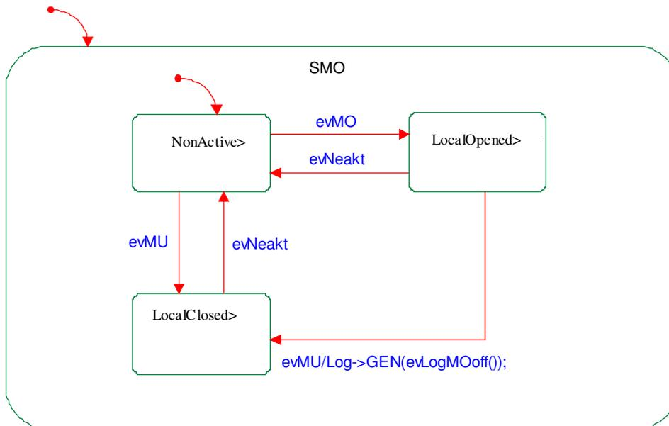
Fig. 2. State Diagram of the class cSmo
