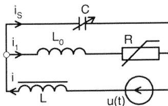
The circuit with one *s*-element is of type  $1 \leq m \leq 5$  if among its closed contours through the *s*-element there is at least one of type  $m$  and none of types less than  $m$ .
