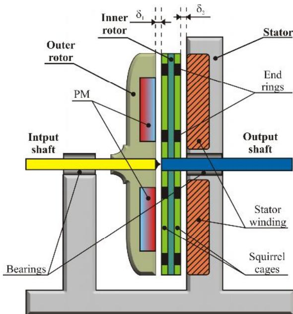
Fig. 2: The AFRC machine in axial cross section.
