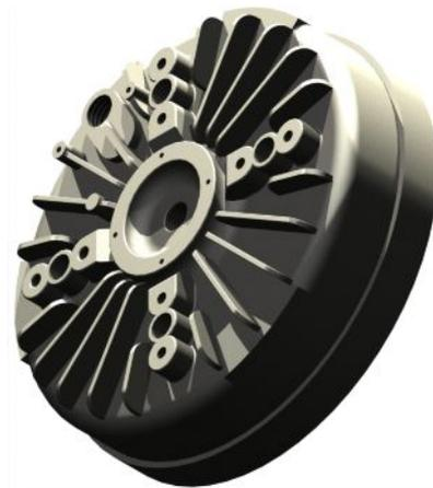
**Fig. 8:** The 3D model of stator housing.
