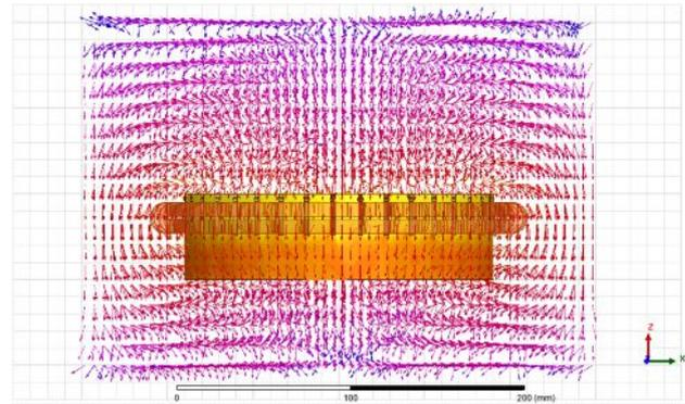
Fig. 12: The vector map of magnetic flux density around the stator pack.
