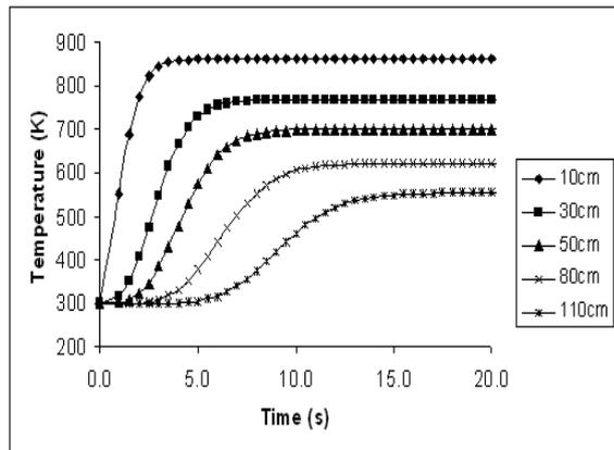
**Figure 9.** CFD Simulated Temperature Profile at Inlet of Catalytic Converter at Position 10 cm, 30 cm, 50 cm, 80 cm and 110 cm from Engine Outlet, respectively.
