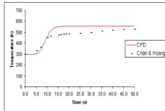
**Figure 8.** CFD Simulated Temperature Profile of the Upstream of Catalytic Converter at 110cm from Engine. Experimental data from Chan and Hoang (1999).
