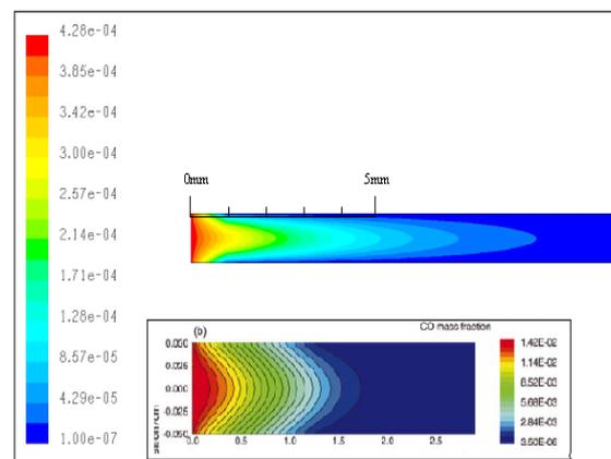
**Figure 11:** CO Mass Fraction Profile inside a Cell at 750K. Inserted diagram at lower right is data from Chatterjee et al. (2001)
