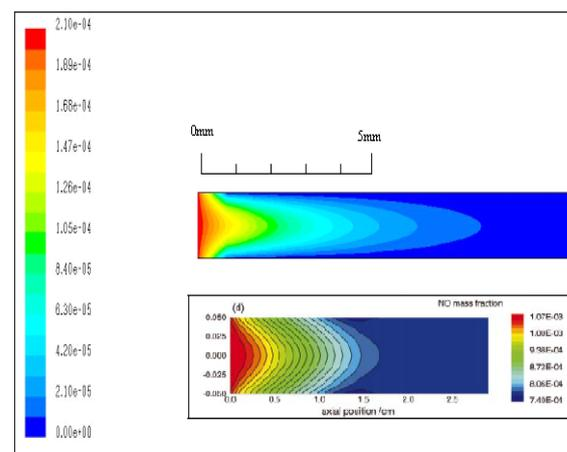
**Figure 10:** NO Mass Fraction Profile inside a Cell at 750K. Inserted diagram at lower right is data from Chatterjee et al. (2001)
