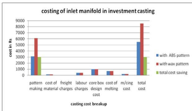
Figure 7 Costing of Inlet Manifold in investment casting (Rs)
