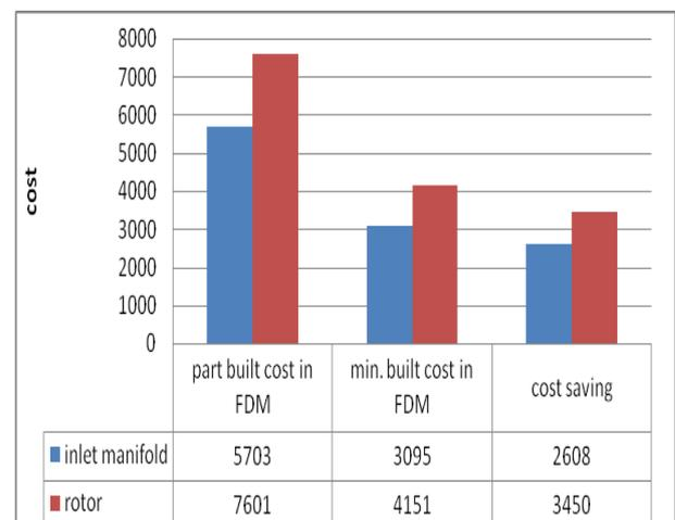
**Figure 5** Cost saving with minimum Parts build cost in FDM
