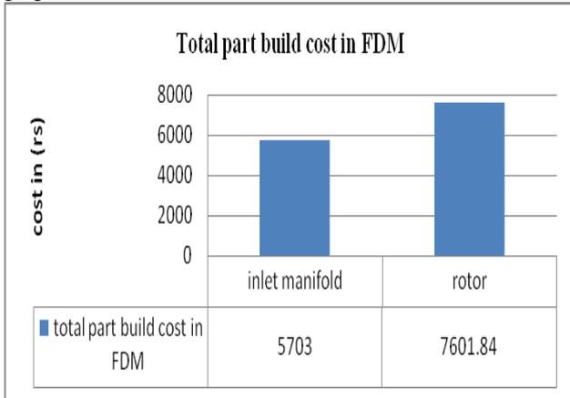
Figure 3 The Part build cost in FDM
