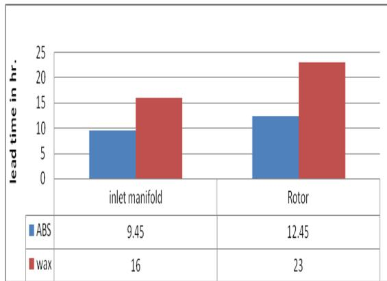
Figure 9 Lead time calculation for patterns
