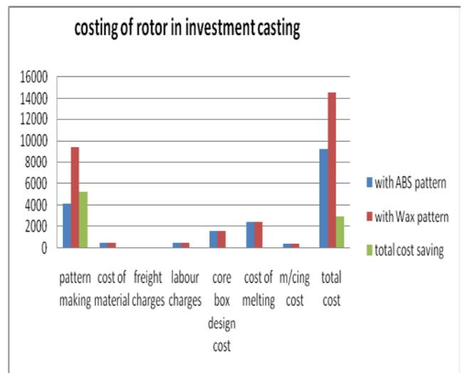
Figure 8 Costing of ROTOR in investment casting
