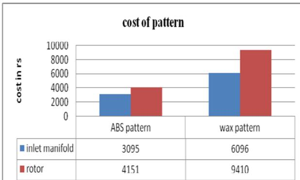
Figure 6 Cost of pattern making with ABS and Wax pattern
