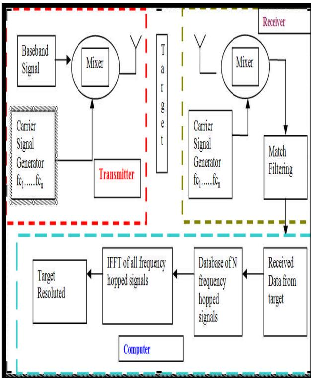
Figure 6. Simulating Model of Frequency Hopping
