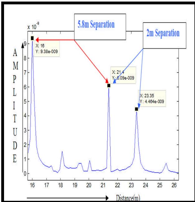
**Figure 10.** Three Targets distinctly resolved when kept at distance of 2m & 5.8m apart with system Bandwidth of 1GHz
