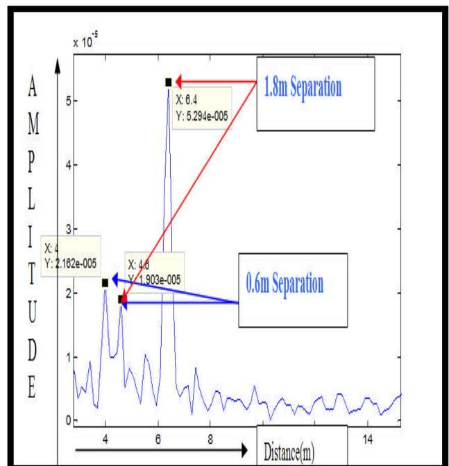
**Figure 15.** Three Targets resolved when kept at distance of 0.6m & 2m respectively apart with system Bandwidth of 1 GHz
