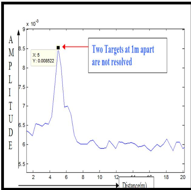
**Figure 12.** Two Targets not resolved when kept at distance 1m apart with instantaneous Bandwidth of 100 MHz
