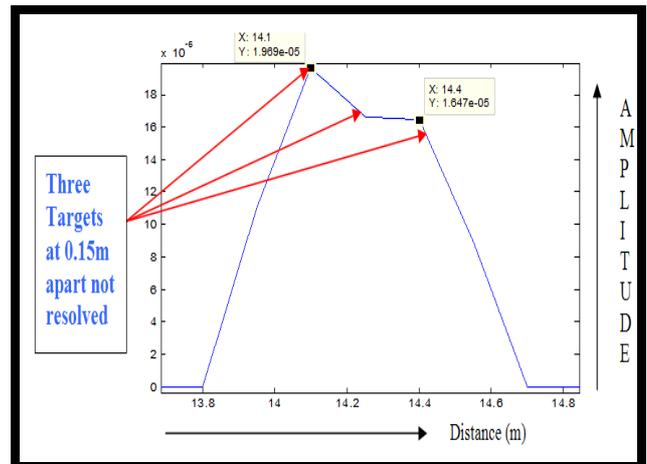
Figure 7. Three Targets not resolved when kept at distance of 0.15m apart with instantaneous Bandwidth of 600 MHz
