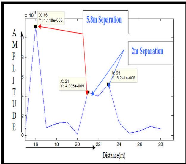
**Figure 9.** Three Targets bit resolved when kept at distance of 2m & 5.8m apart with system Bandwidth of 150 MHz
