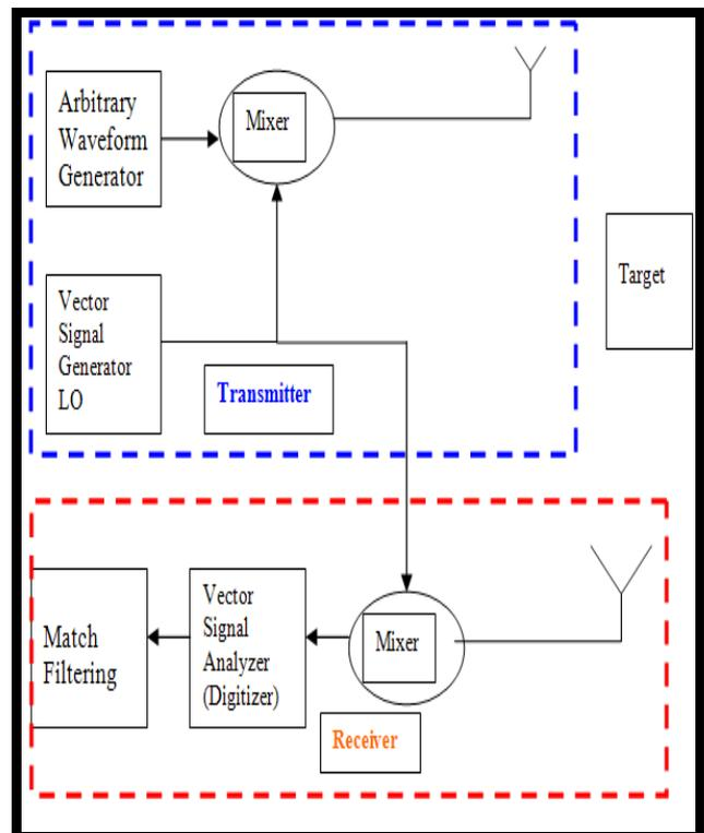
**Figure 11.** Hardware Model of Frequency Hopping
