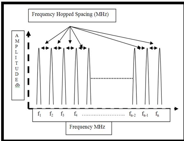
Figure 5. Frequency Hopped Model
