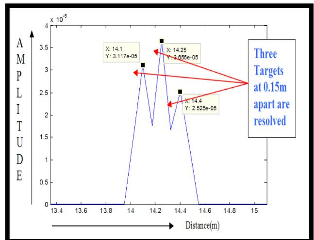
Figure 8. Three Targets resolved when kept at distance of 0.15m apart with instantaneous Bandwidth of 1 GHz 1000MHZ
