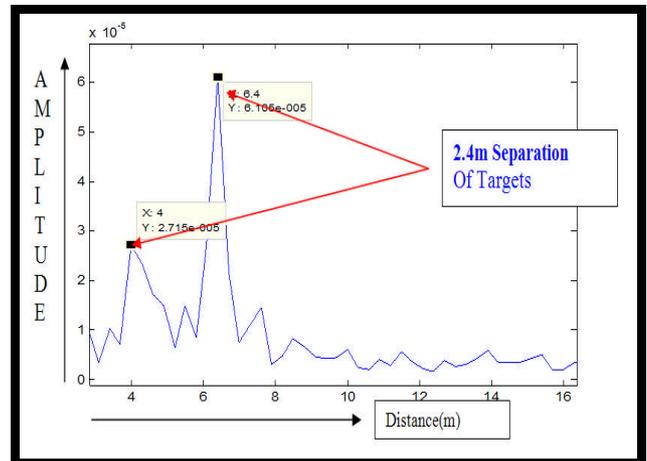
**Figure 14.** Three Targets not resolved when kept at distance of 0.6m & 2m respectively apart with system Bandwidth of 500 MHz
