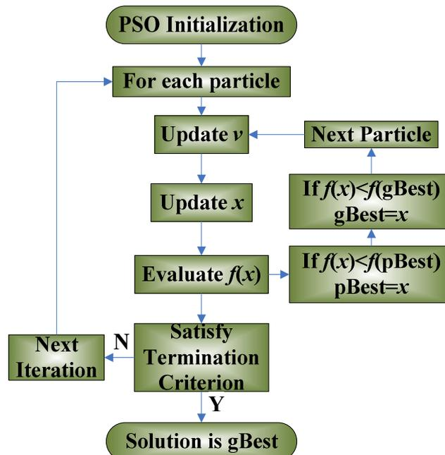
Fig. 2 Flow chart of the PSO algorithm
