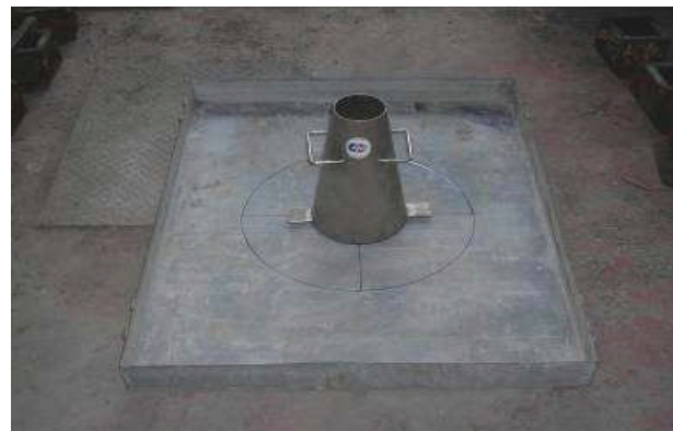
Fig. 1: Slump Flow Test
