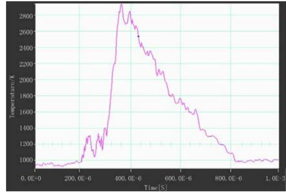
**Figure 6.** The true temperature curve of the output flame of the electric igniter
