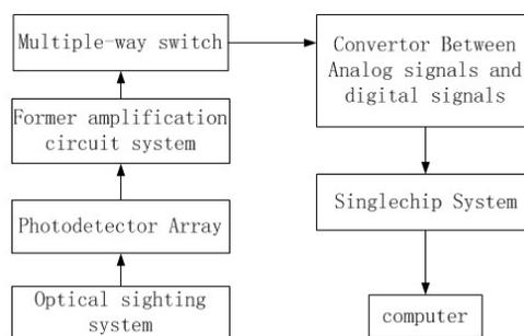
Figure 1. The multi-spectral radiation thermometer
