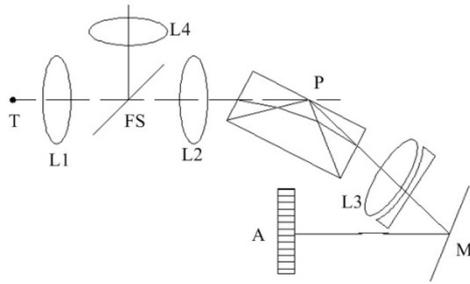
**Figure 2.** The optical system of the multi-spectral radiation thermometer
