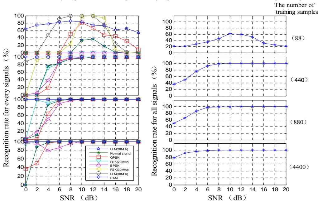
Figure 3. The recognition rates for every signal and all signals varying with different SNR
