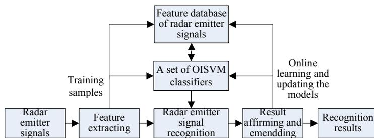
Figure 1. The scheme of radar emitter signal recognition method based on OISVMs.
