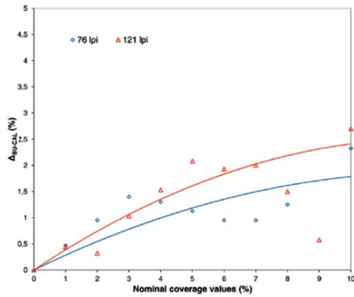
Figure 8. Results of coverage values in lighter tones after application of the bump-up curve for the 76 lpi and the 121 lpi screen ruling
