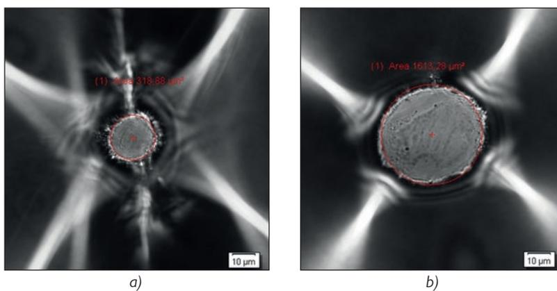
Figure 10. Images of the printing plate sample at 5% coverage value for the 121 lpi screen ruling after corrections with a) application of the calibration curve; b) application of the bump-up curve
