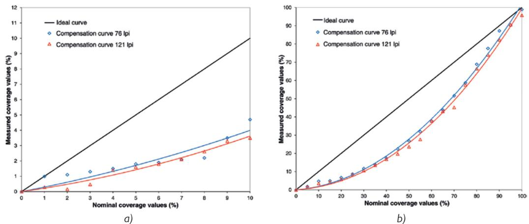
Figure 11. Comparison of the results of the compensation curves for the 76 lpi and the 121 lpi screen ruling a) nominal coverage values from 1% - 10%; b) nominal coverage values from 1% - 100%
