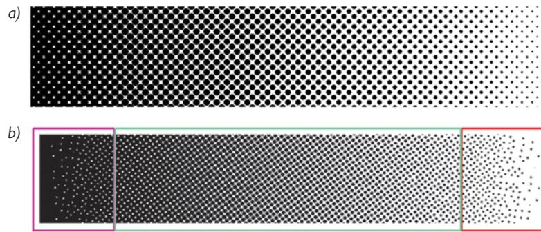
Figure 3. Examples of screen type in flexography – a) AM screen, b) hybrid screen
