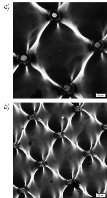
Figure 5. Microscopic images of flexographic printing plate sample on 3% nominal coverage value at 200 $\times$  magnification after application of the calibration curve (without the bump-up) for a) the 76 lpi and b) the 121 lpi screen ruling
