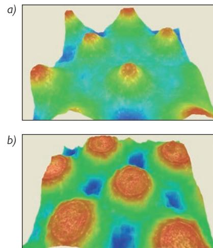
Figure 4. 3D view of flexographic printing plate at a) 5% and b) 50% nominal coverage value, 76 lpi
