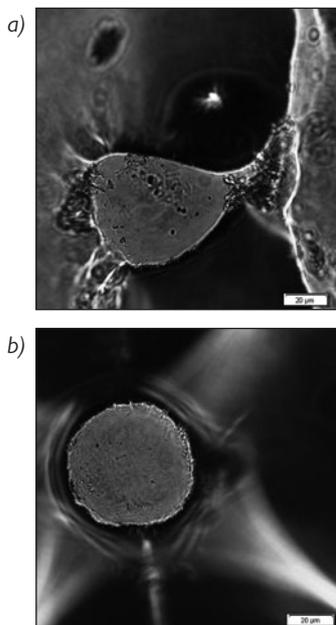
Figure 2. Microscopic images of printing element in lower coverage values;
