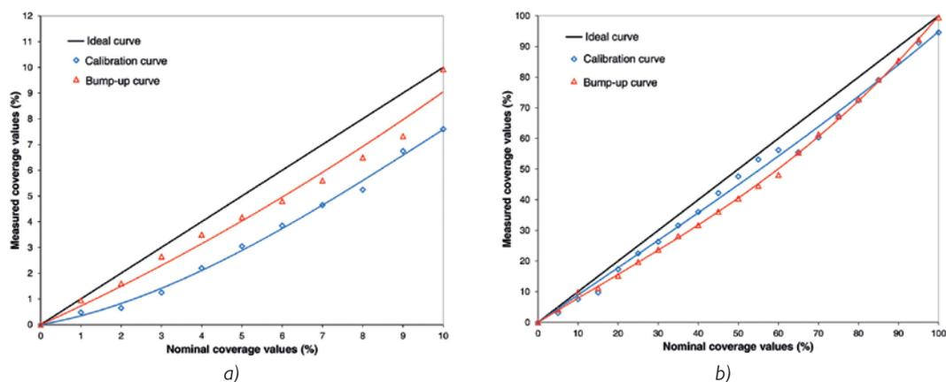
Figure 6. Comparison of the results of the calibration and the bump-up curve for the 76 lpi screen ruling a) coverage values from 1% - 10%; b) coverage values from 1% - 100%
