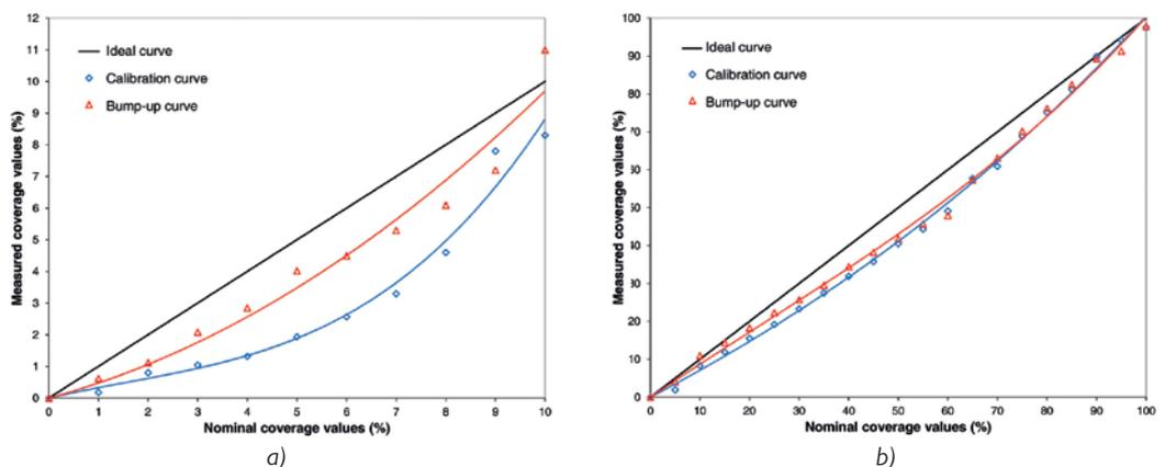
Figure 7. Comparison of the results of the calibration and the bump-up curve for the 121 lpi screen ruling a) nominal coverage values from 1% - 10%; b) nominal coverage values from 1% - 100%
