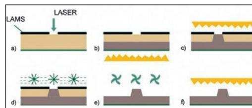
Figure 1. Production of photopolymer printing plate with LAMS; a) laser ablation; b) back-exposure; c) main exposure; d) chemical and mechanical developing; e) drying; f) post-exposure (UV-A, UV-C).
