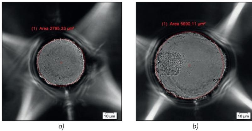
Figure 9. Images of flexographic printing plate sample at 5% coverage value for the 76 lpi screen ruling a) after application of the calibration curve; b) after application of the bump-up curve
