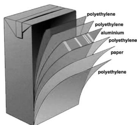
Figure 2. Wall layers of Tetra Pak aseptic packaging.
