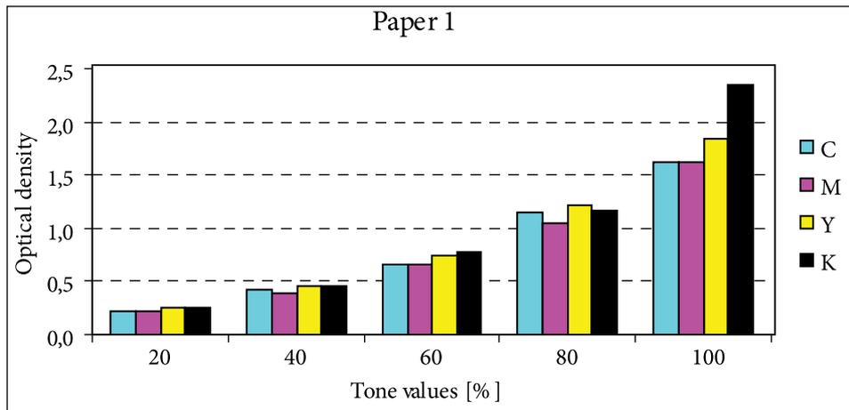
Figure 1: Optical density of CMYK prints at Paper 1.
