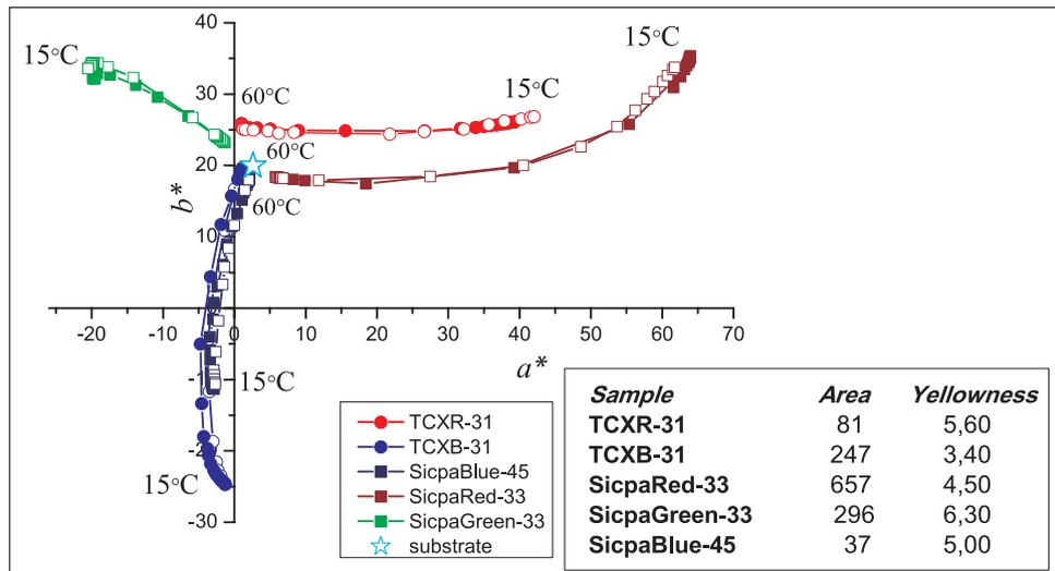
Figure 3. Colour trajectories in the ( $a^*, b^*$ ) plane of CIELAB colour space as obtained for five TC samples at heating (full signs) and cooling (open signs). The value of the applied bare paper substrate (OBA free gloss coated paper, 150 g/m<sup>2</sup>) is marked with a star. The area of the surface between two trajectories in the CIELAB colour space is shown in the key (Area) (quadratic CIELAB units). The degree of discoloration (Yellowness) is also specified (in CIELAB units).
