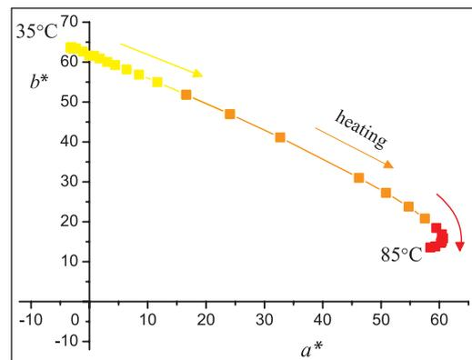
Figure 4. Changing of CIELAB values of irreversible Yellow-to-red TC sample in ( $a^*, b^*$ ) plane at heating.
