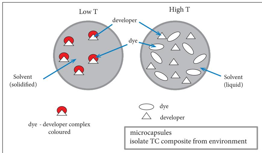
Figure 1. Schematic representation of leuco dye-developer solvent composite system
