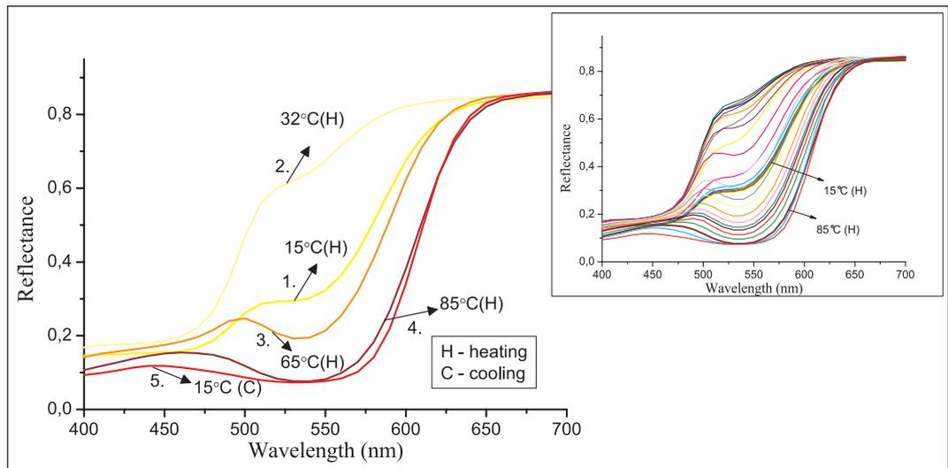
Figure 7. Reflectance spectra of irreversible TC ink printed on top of the red TC ink (H signs – temperature, in °C, reached by heating, C signs – temperature, in °C, reached by cooling).
