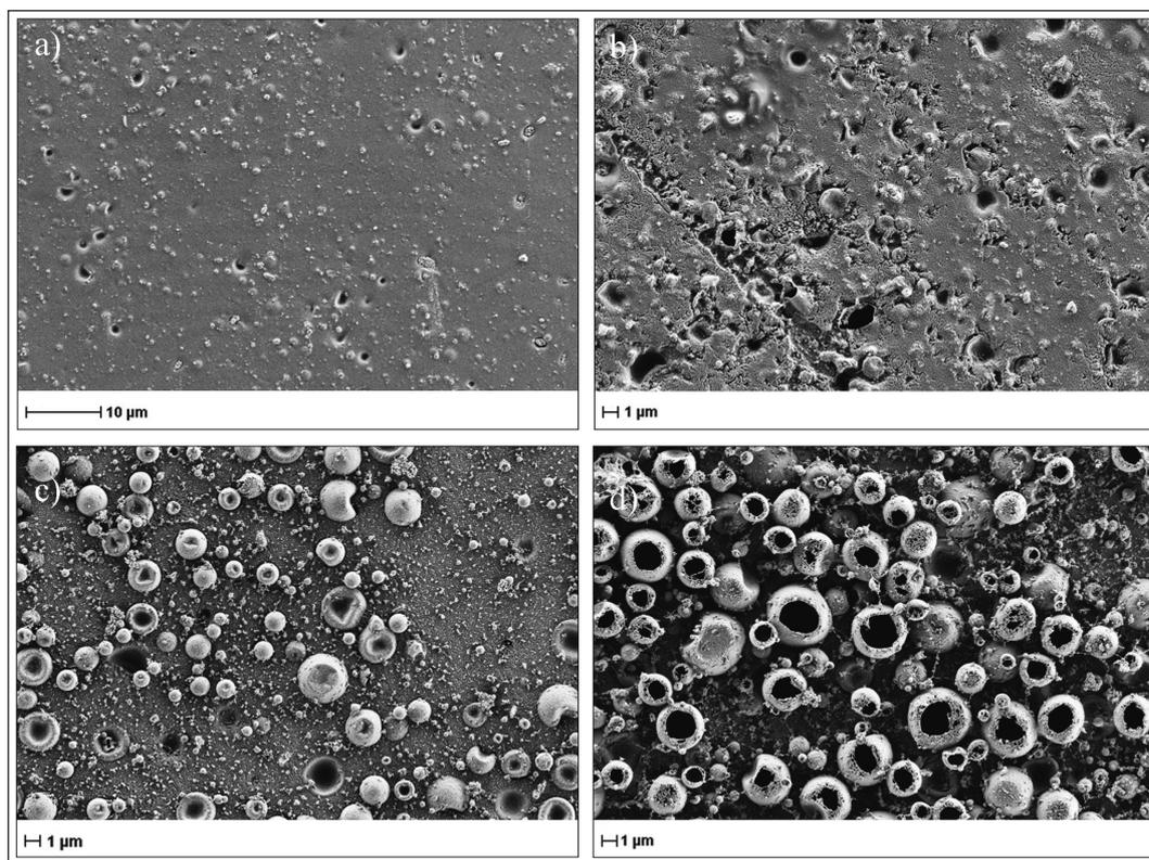
Figure 9. SEM micrograph of the TC sample SicpaGreen-33 without oxygen plasma treatment (a), after 30s exposure to oxygen plasma (b), after 60s exposure to oxygen plasma (c) and after 120s exposure to oxygen plasma (d).
