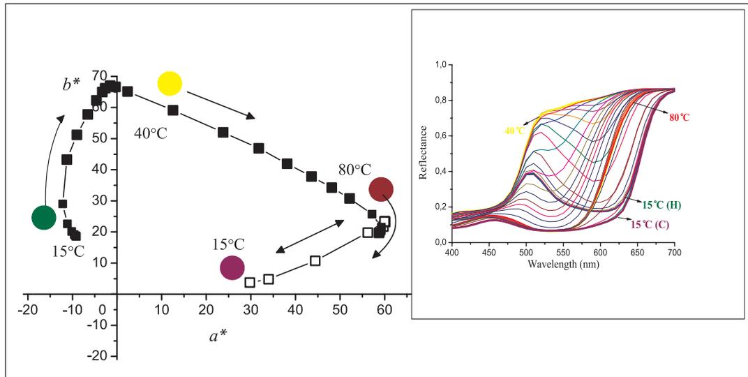
Figure 8. Changing of CIELAB values of irreversible TC ink printed on top of the blue thermochromic ink in ( $a^*$ ,  $b^*$ ) plane at heating, irreversible change, (solid signs) and cooling, reversible change, (open signs). Small figure represents reflectance spectra of irreversible TC inks printed on top of the blue TC ink.
