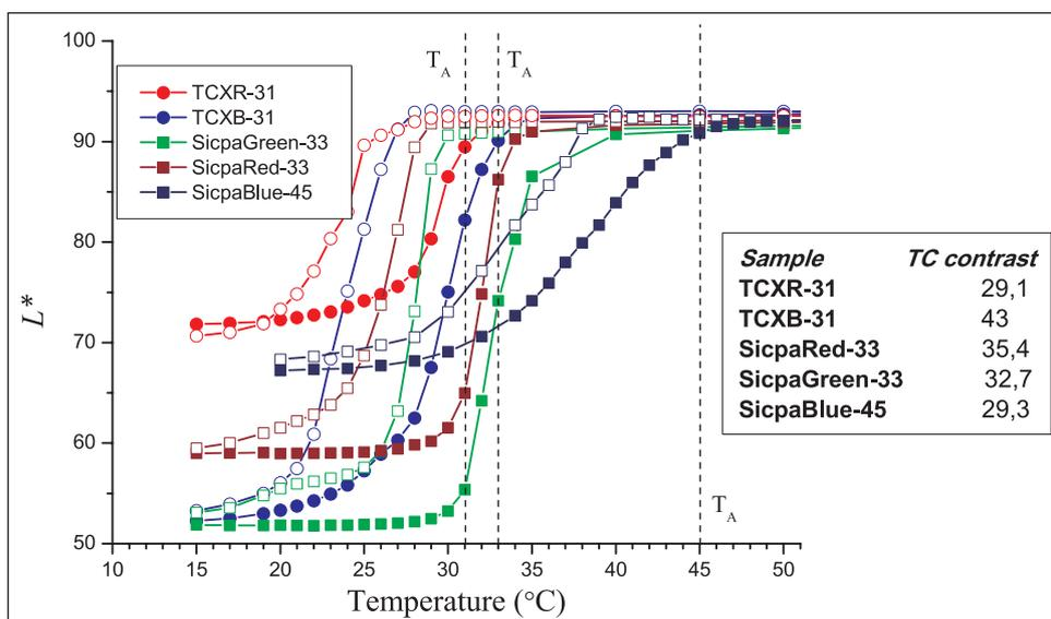
Figure 5. Colour hysteresis of TC samples. CIELAB colour values as a function of temperature for five TC samples: TCXR-31, TCXB-31, SicpaRed-33, SicpaGreen-33 and SicpaBlue-45 at heating (full signs) and cooling (open signs). Samples with similar layer thickness were evaluated. Efficiency of colour change is expressed by TC contrast, the total colour difference between totally coloured and discoloured states and is given in the key (in CIELAB units).
