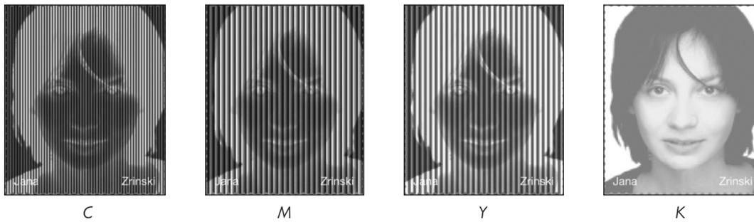
Figure 7. CMYK channels of a picture that has undergone CMYKIR separation
