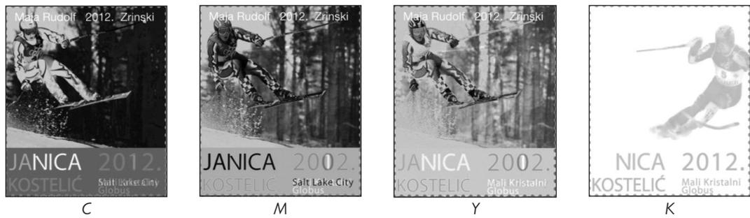
Figure 5. Single channels of a picture that has undergone CMYKIR separation
