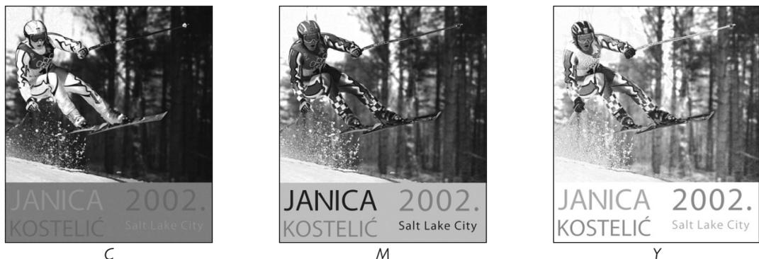
Figure 3. Conversion phase of the conventional CMYK image into CMY with  $K = 0$
