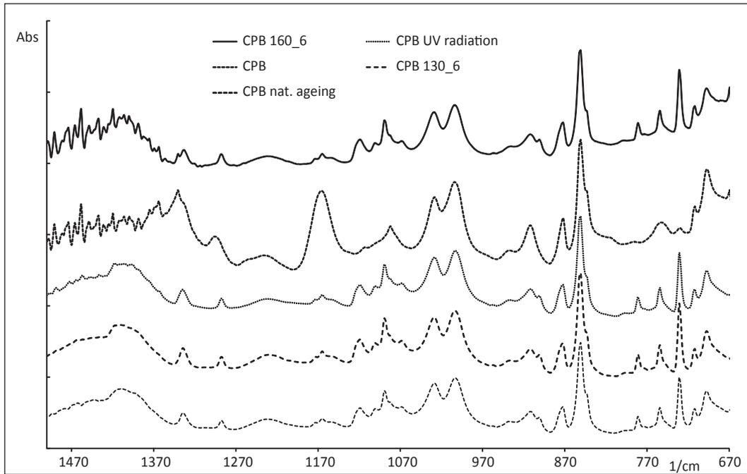
Figure 9. IR spectra of coated samples printed with Process Blue ink before and after ageing (spectra are shifted in absorbance for clarity)
