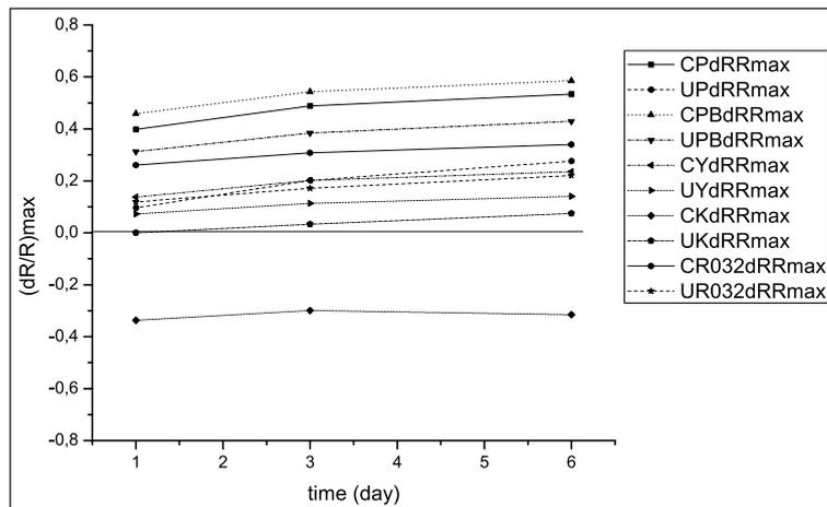
Figure 7. Maximum relative reflectance differences at specific wavelength,  $(dR/R)_{\max}$  for all measured samples after they had been exposed to heat in the oven at 130 °C for one, three and six days.
