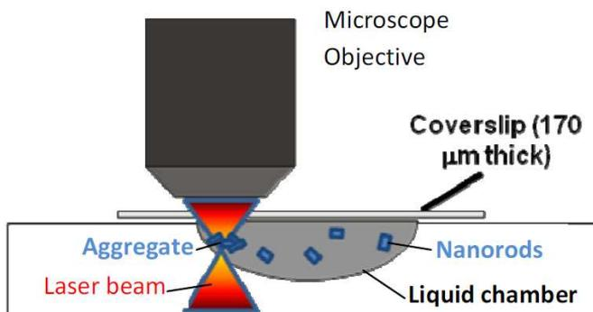
**Figure 1.** Schematic of the setup showing the nanorods aggregation under the laser beam.
