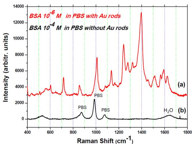
**Figure 2.** (Red line) SERS spectrum of buffered BSA molecules at 1 mM taken after the formation of the nanorods aggregates. (Black line) Raman spectrum of buffered BSA solution at 100mM without the addition of nanorods. The spectra are offset for clarity.
