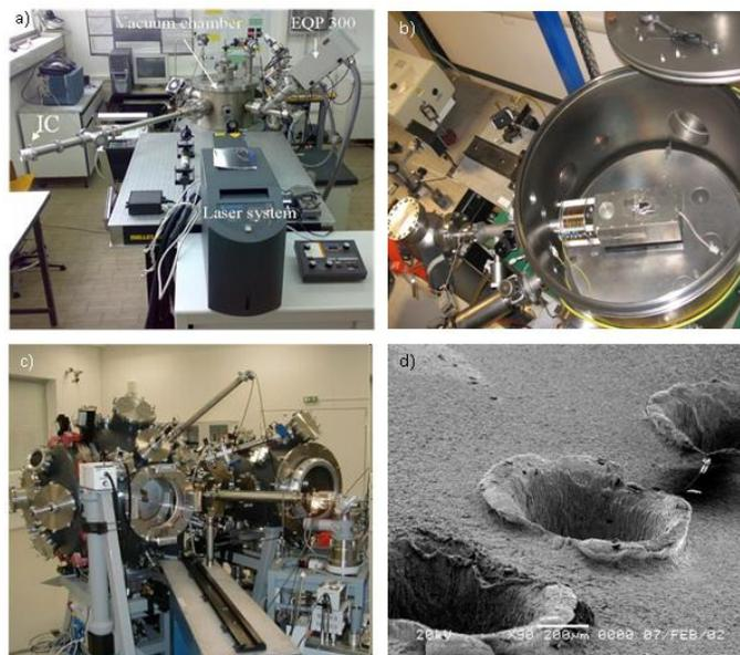
**Figure 1.** (a) “Laboratorio di Fisica dei Plasmi Laser” of the Physics Department of Messina University; (b) post-ion acceleration set-up at INFN-LNS of Catania; (c) International Laboratory PALS of Prague; (d) SEM photo of typical craters in a Cu thick target irradiated by the laser pulses at PALS.
